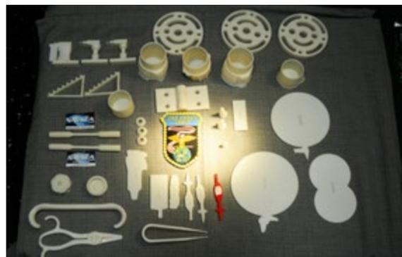
Test specimens and sample specimens fabricated aboard USS Essex (LHD 2) included tensile tests, tested by Naval Surface Warfare Center, Carderock Division, and geometric, dimensional and tolerance specimens, tested by Naval Surface Warfare Center, Corona. Sample specimens were designed and fabricated aboard Essex with support from the Naval Postgraduate Dental School. (U.S. Navy photo provided by USS Essex public affairs/Released)
