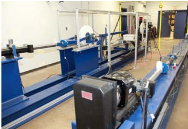
The Tow Cable Test Site (TCTS) incorporates two separate test fixtures - (foreground) the tension test fixture capable of exciting loads up to 25,000 pounds and the Bend Over Sheave (BOS) fatigue test fixture, which utilizes a belt driven actuator to drive a tow cable around a set of two fixed sheaves while under tension in order to assess the bending fatigue life of a cable (U.S. Navy photo by Public Affairs Specialist Joseph Battista/Released).
