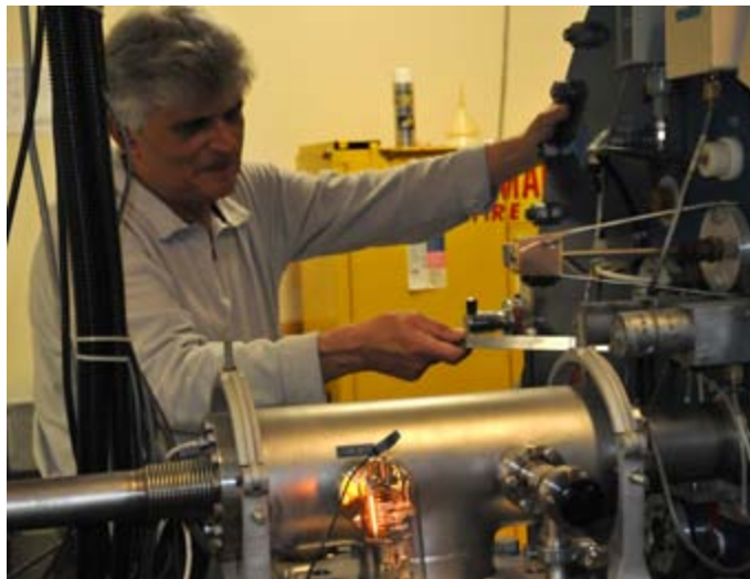
Dr. Noel Guardala (above) checks on the gas stripper control system which is vital to the production of a 2 MeV C beam, essential to producing kinematically compressed fast neutrons (U.S. Navy photo by Nicholas Malay/Released).
