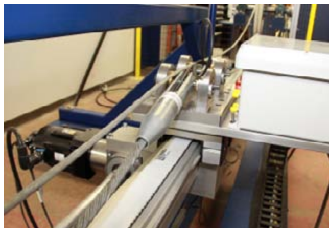
The Bend Over Sheave (BOS) fatigue test fixture utilizes a belt driven actuator to drive a tow cable around a set of two fixed sheaves while under tension in order to assess the bending fatigue life of a cable (U.S. Navy photo by Public Affairs Specialist Joseph Battista/Released).
