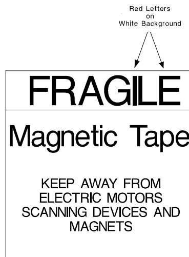
FIGURE B.2. Example of a warning label.
