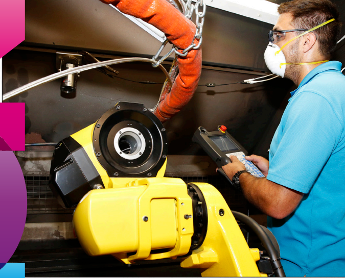
LEFT TO RIGHT: Machinist Sean Schuffert prepares a cold spray booth to repair a critical part for the USS George H.W. Bush (CVN 77); Machinists Sterling Slaughter and Sean Schuffert set up a cold spray booth to cold spray a part for Norfolk Naval Shipyard (NNSY).
