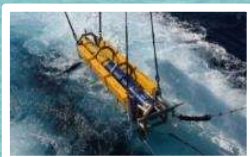
Knifefish UUV Block 0 • Bottom & Buried Mine Hunting
