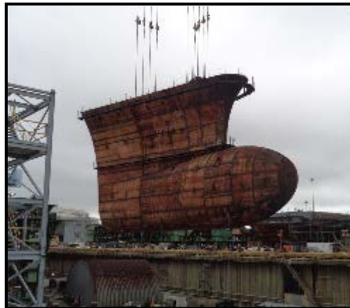
Bulbous-Bow section being lowered to primary ship structure
