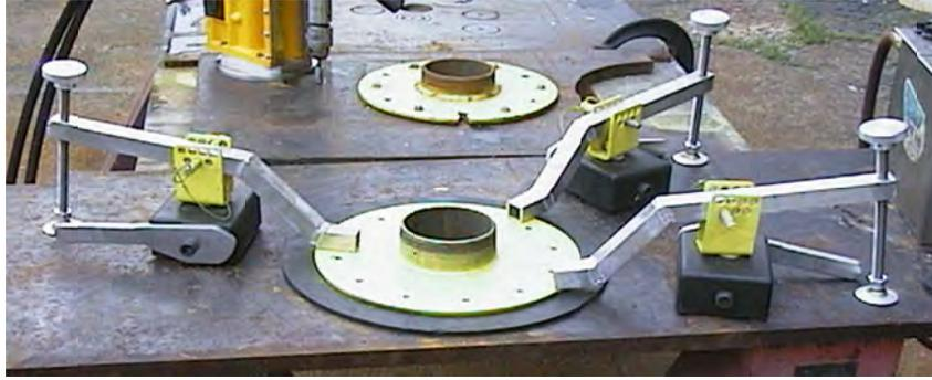
Figure 5-5. Hot Tap Flange Held in Place with Magnets
