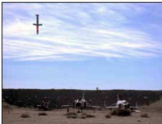
Tomahawk missile executed a planned Variable Dive Maneuver inert warhead impact against aircraft revetment target. U.S. Navy photo.
