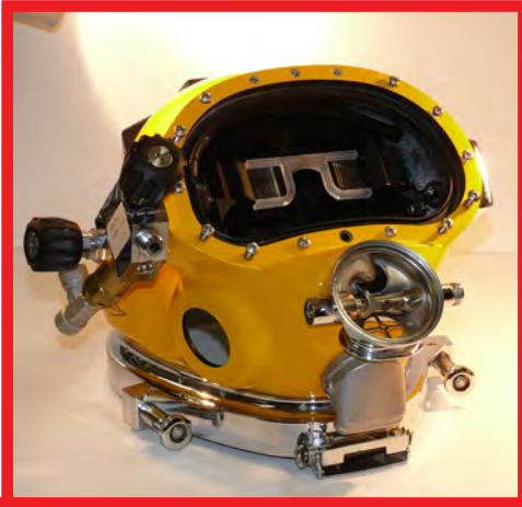
Prototype of the Divers Augmented Vision Display (DAVD) positioned within a dive helmet. U.S. Navy Photo by Richard Manley (RELEASED)
