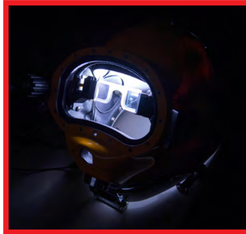
Lab simulation view of an augmented reality image of an airplane through the Divers Augmented Vision Display (DAVD). Divers Augmented Vision Display (DAVD). U.S. Navy Photo by Richard Manley (RELEASED)
