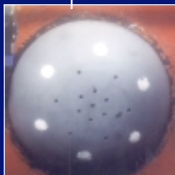
Typical ICCP reference cell (9-Inch Diameter).
