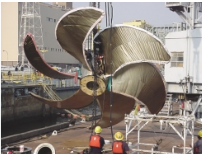
Preparing to install new propeller on USS SUPPLY AOE 6. Left to right: BM1(DV) Lafever and Mr. Tony Kriedler.
