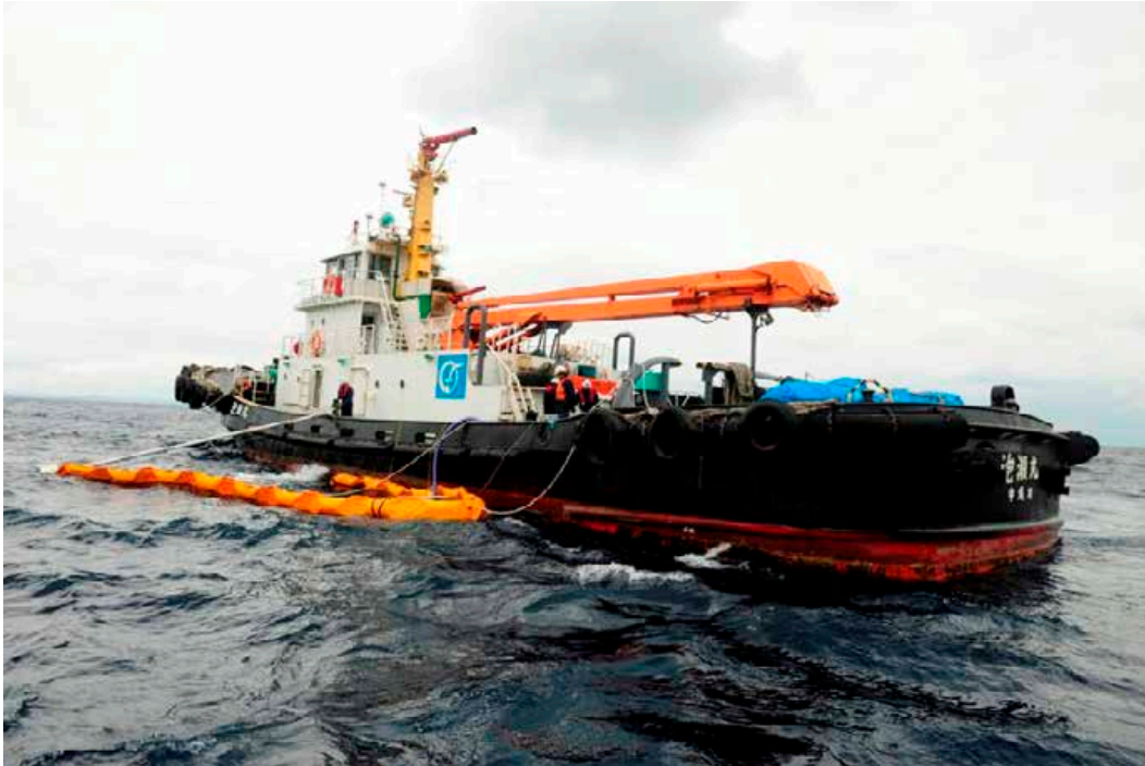
Figure 5-1. During the refloating phase, oil response vessels were on the scene in the advent of a fuel spill. This is the support tug Awase Maru with a boom and skimmer deployed demonstrating their readiness should a spill occur.
