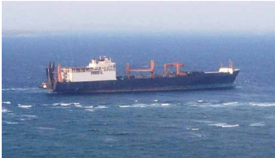
Figure 1-1. USNS KOCAK grounded on Ufubishi Reef, Okinawa, Japan. Reef shoal is marked by breaking waves in the foreground.
