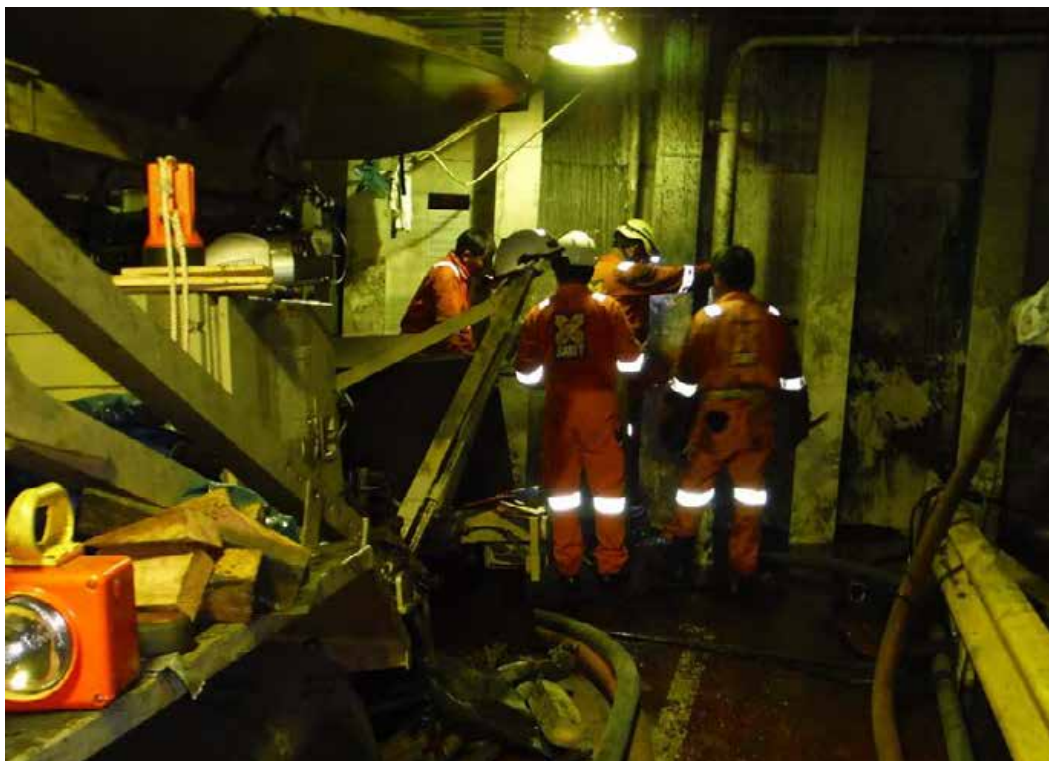
Figure 3-9. SMIT salvors assessing leak rates in Hold 3A.
