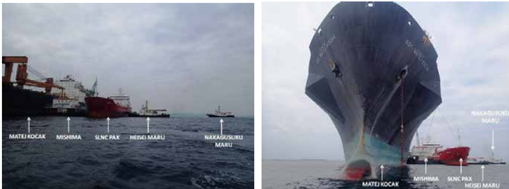
Figure 3. Overview of fuel lightering operations, where MISHIMA barge is used as a ‘fender’ between MATEJ KOCAK and SLNC PAX during fuel lightering operations. Tugs HEISEI MARU and NAKAGUSUKU MARU are onsite for salvage operations. Note port anchor underfoot. (2 February 2015).
