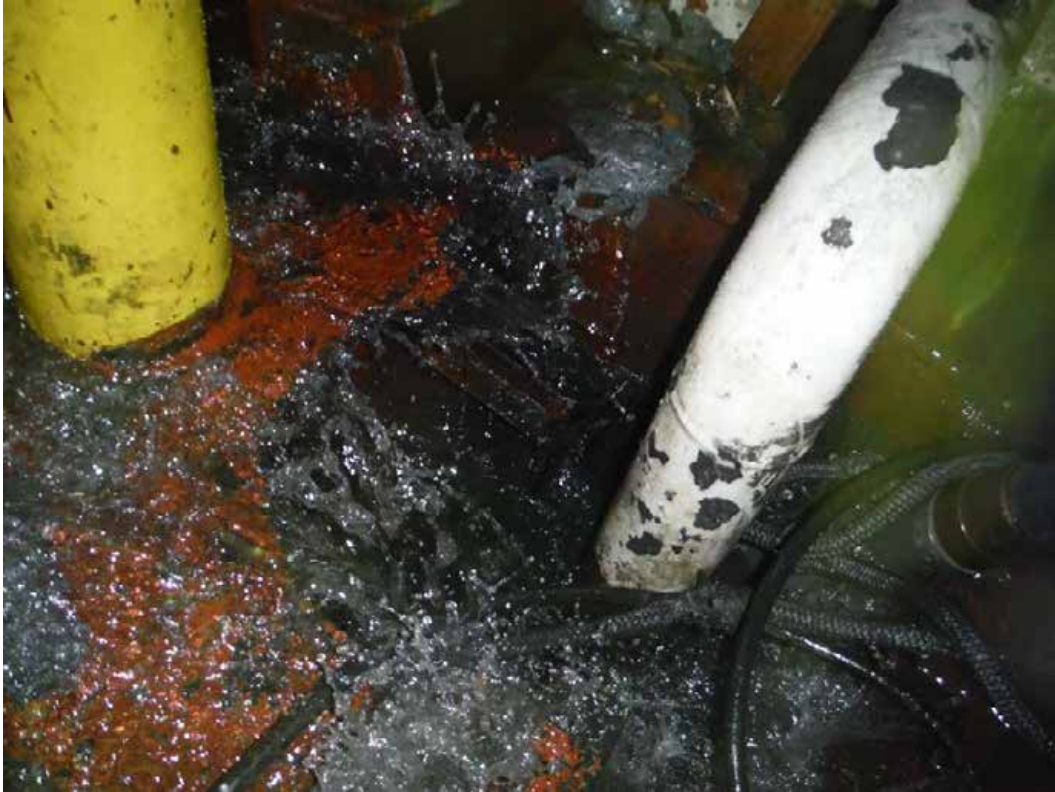
Figure 3-5. Seawater freely flowing from sump in Hold 3A.
