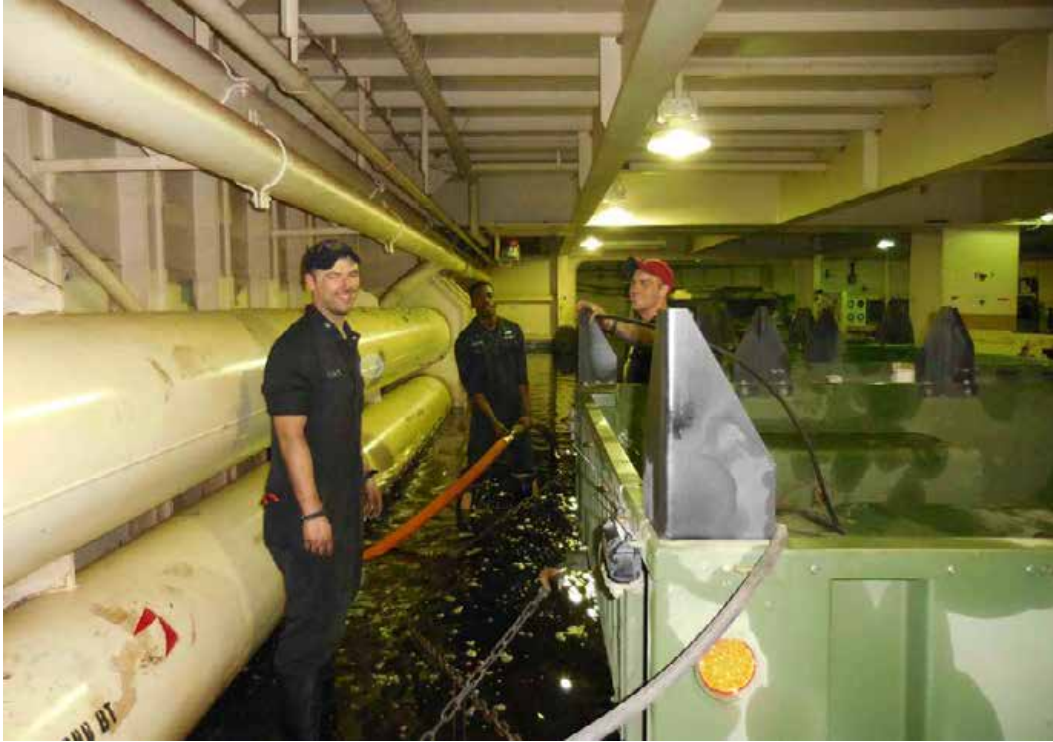
Figure 3-6. USS BONHOMME RICHARD Damage Control Team members conducting dewatering operations.
