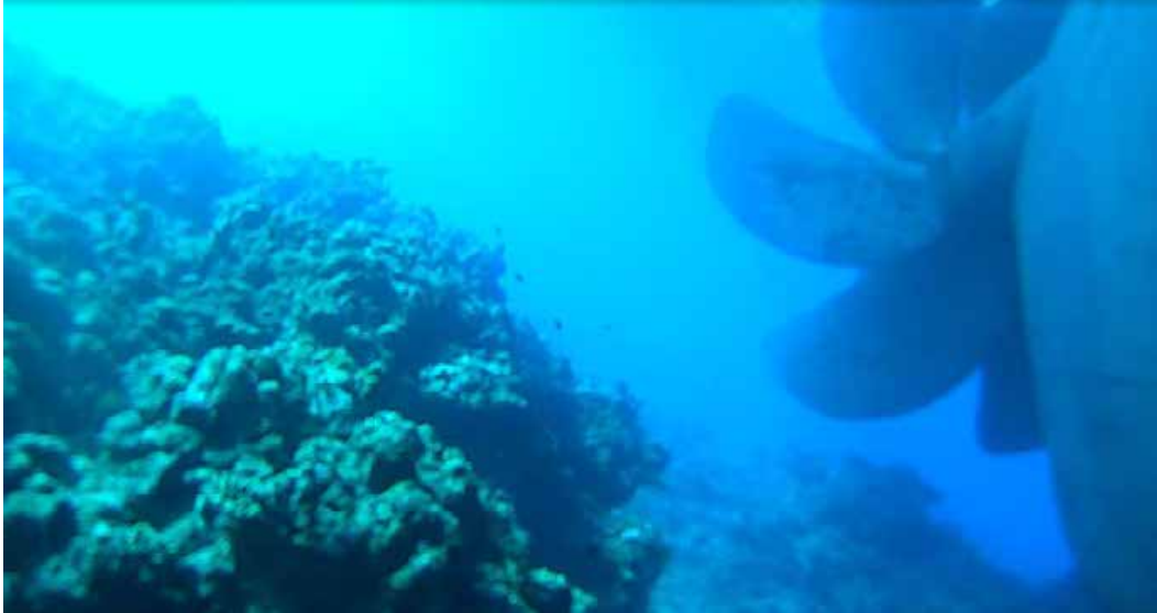
Figure 3-13. Propeller clearance to reef from 29 January dive survey video.
