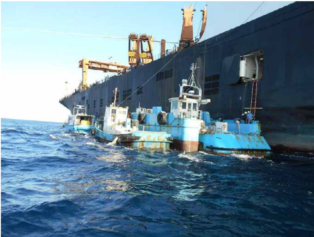
Figure 3-4. KOCAK grounded with U.S. Navy Commander Fleet Activities Okinawa (CFAO) White Beach waste oil containment barge, Kanto 18, alongside for collection of oily bilge water.
