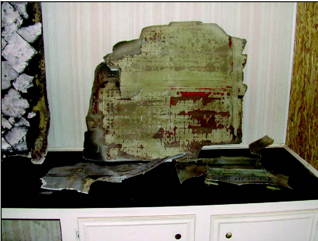
Figure 3-14. Actual Shuttle Pieces Used as Test Targets.
