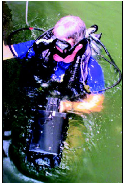
Diver utilizing LIMIS system
