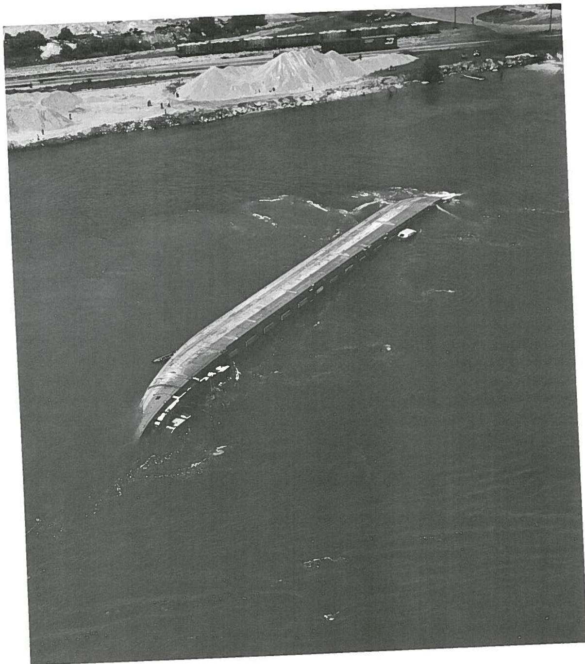
Morning after collision, wreck was already beginning to settle and break up. Water poured in through cargo hold hatches and at point of impact. Extensive flooding, plus rapid scouring of river bottom beneath bow region (right), created severe stresses on hull. SMITH STILL INTACT BUT VULNERABLE TO FURTHER DAMAGE
