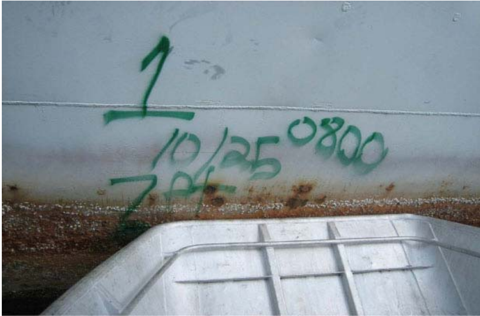
Figure 7. Location 1 Outboard Shell Plate. Readings were taken both above and below the rust/scale line.
