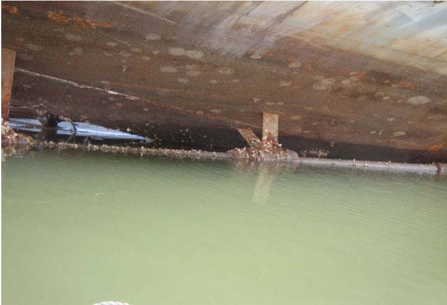
Figure 13. Location 6 and 7 would forward of this picture to the right side. Location 8 is just outboard of the center strut bearing hull attachment and location 9 is midway between the strut bearing and the prop near the upper left padeye left in this picture. Note – shaft angle is known so this photo provides good evidence of the vessel's trim.
