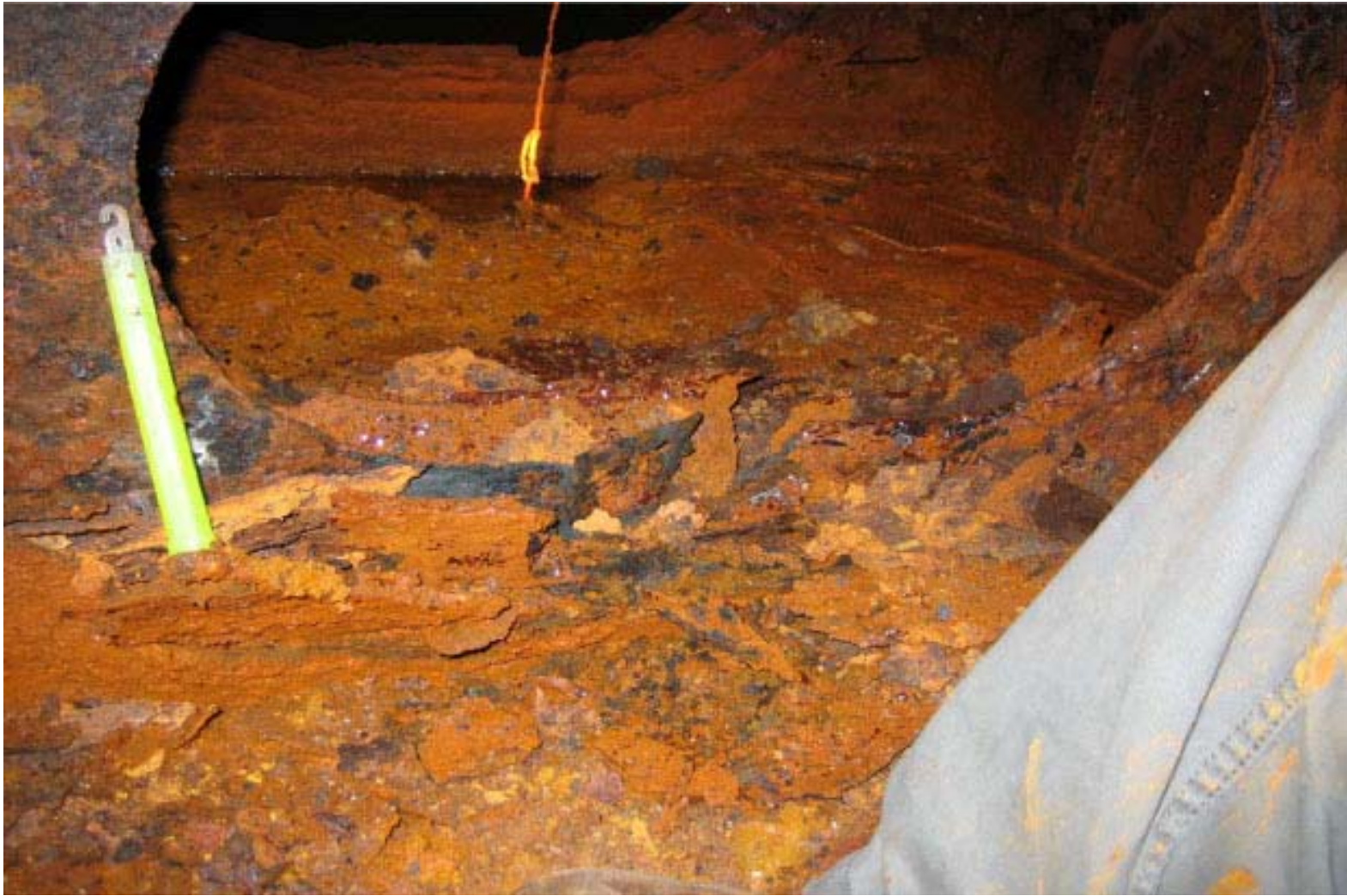
Figure 1. Longitudinal structural support frame in port engine space bilge shows rust and scale deterioration with heaviest deterioration along shell plate interface. Typical of most frames (transverse frames, longitudinal frames and many intercostals in the engine room spaces.
