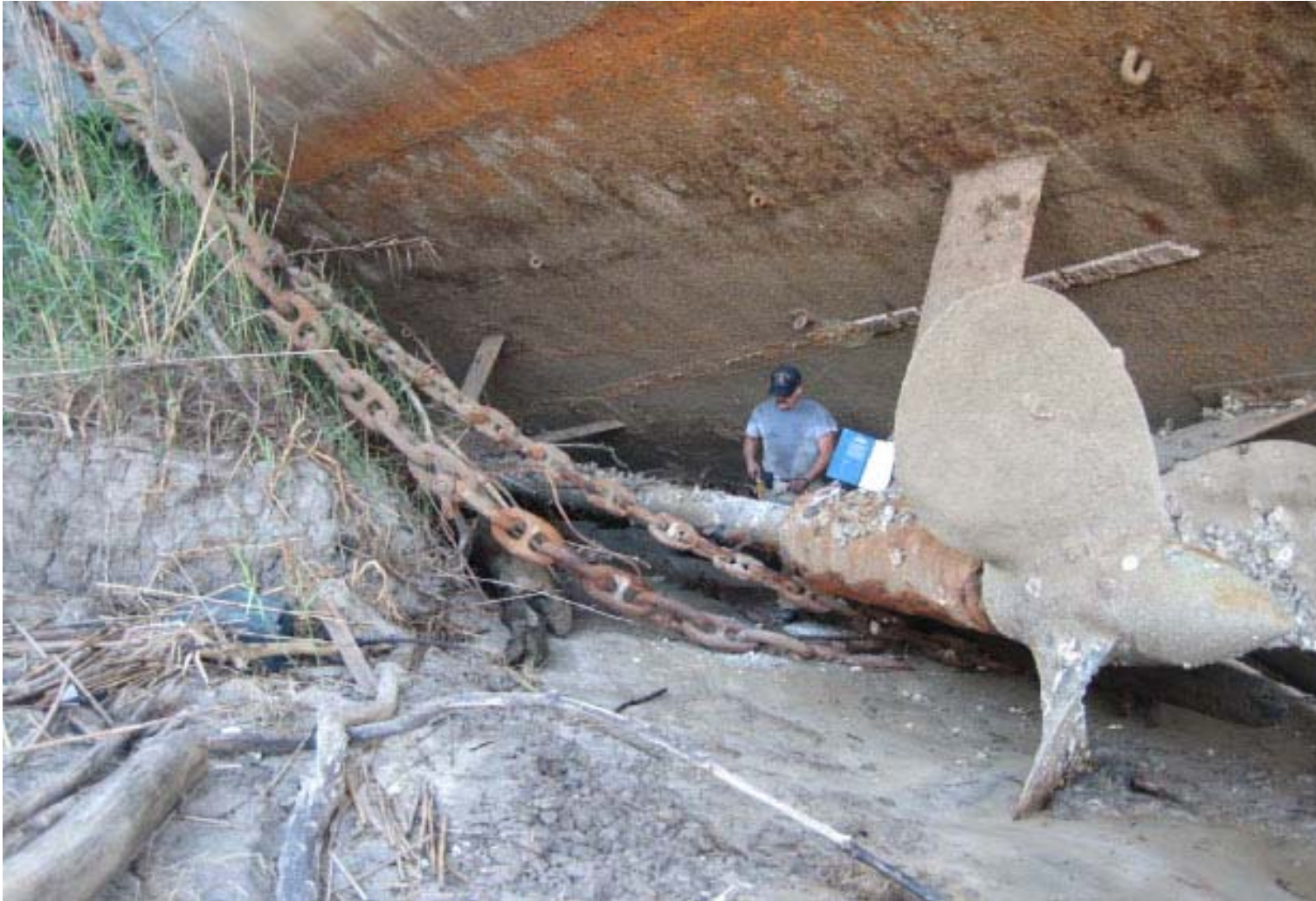
Figure 14. Hull UT readings 10 and 11 were taken on the port stern. Number 10 was located to the right of the shaft next to where the worker is shown in this photo. Number 10 is also where the hole was created in the weld seam. Location 11 is further forward near the strut bearing.
