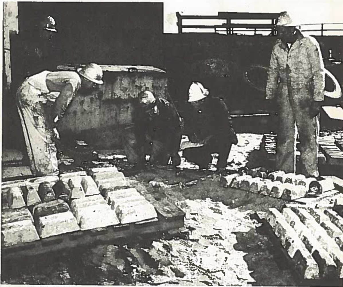
FIGURE 6.—Arrangements for testing to determine coefficient of friction.
