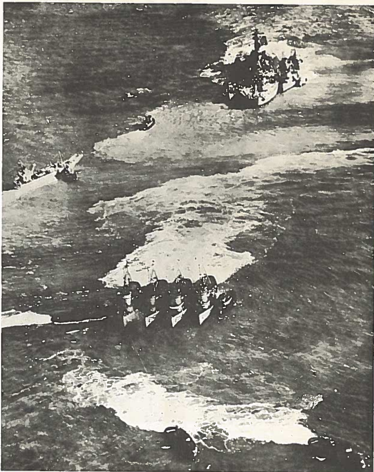
Water churned up by straining tugs during unsuccessful pull attempt on 20 January. Involved were 4 ATF's, 2 ASR's, 2 ARS's, 2 ATA's, and a number of small YTB type tugs. Approximately 8,000 tons, mostly fuel, had been removed from the Missouri and considerable dredging along each side had been accomplished.
