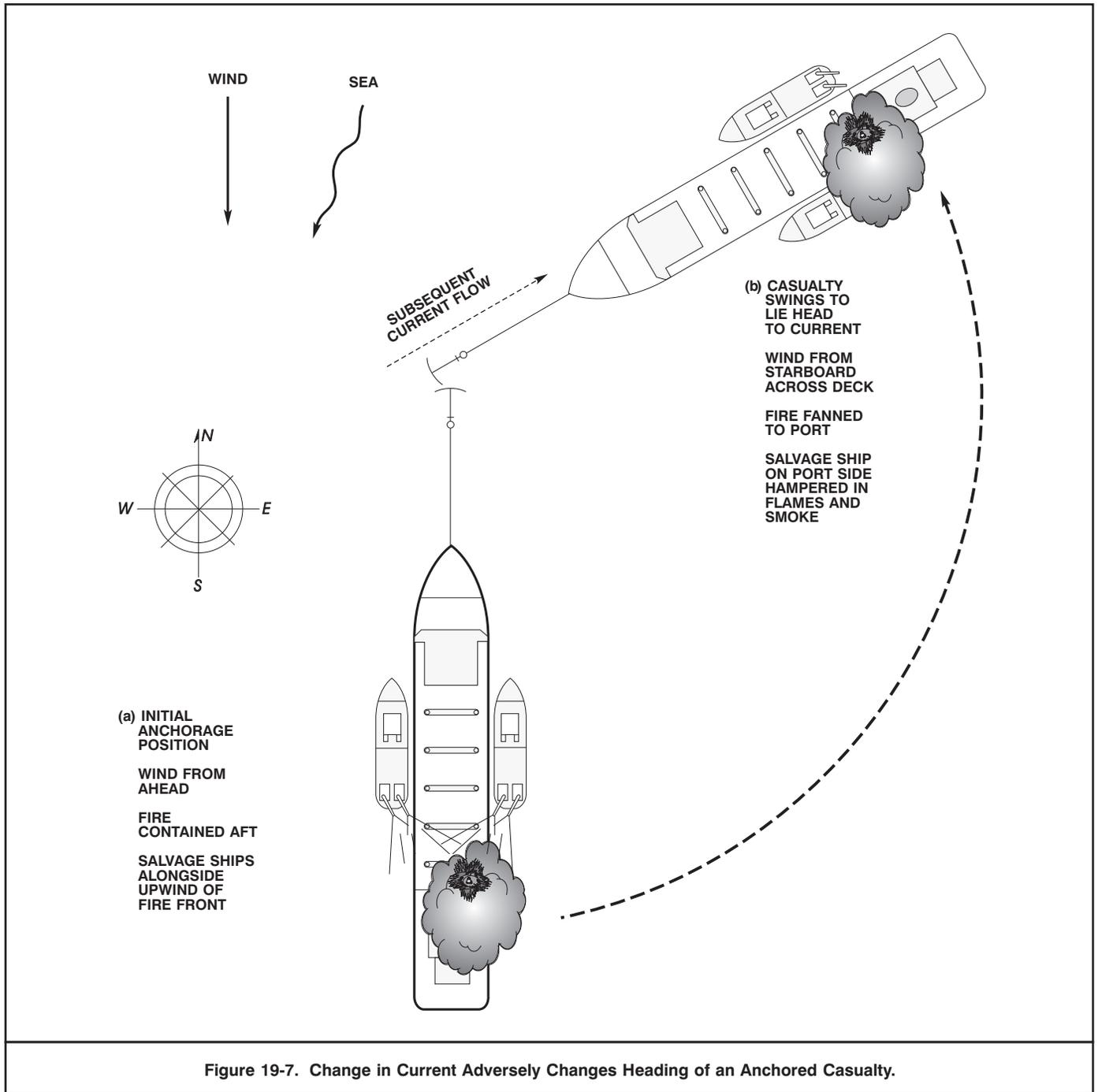
Figure 19-7. Change in Current Adversely Changes Heading of an Anchored Casualty.
