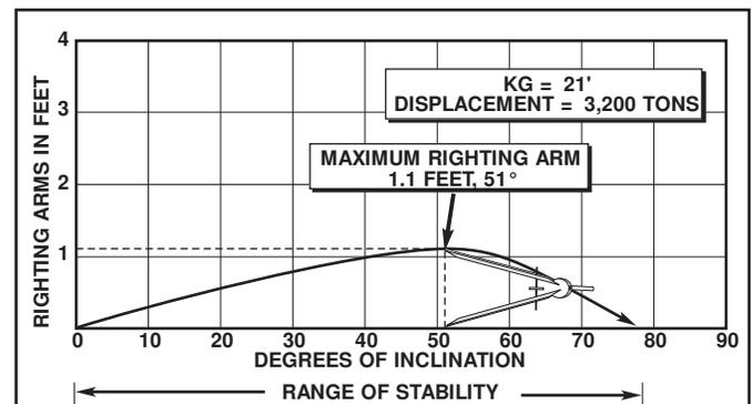
Figure 4-7. Corrected Statical Stability Curve.
