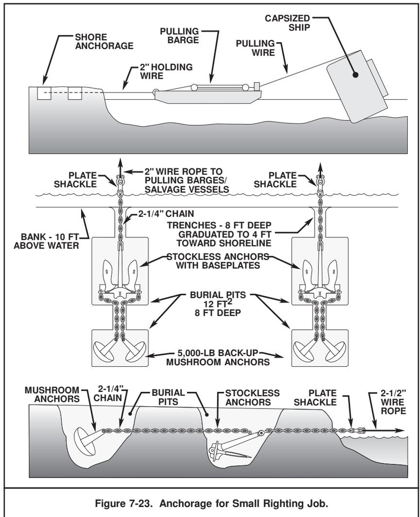
Figure 7-23. Anchorage for Small Righting Job.
