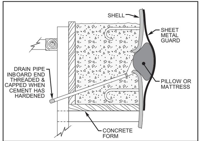
Figure 10-30. Typical Drain Pipe Installation.
