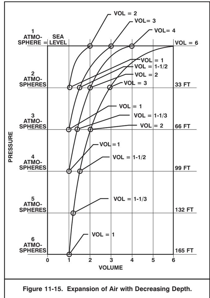
Figure 11-15. Expansion of Air with Decreasing Depth.
