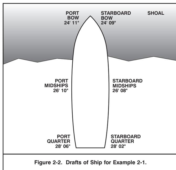
Figure 2-2. Drafts of Ship for Example 2-1.
