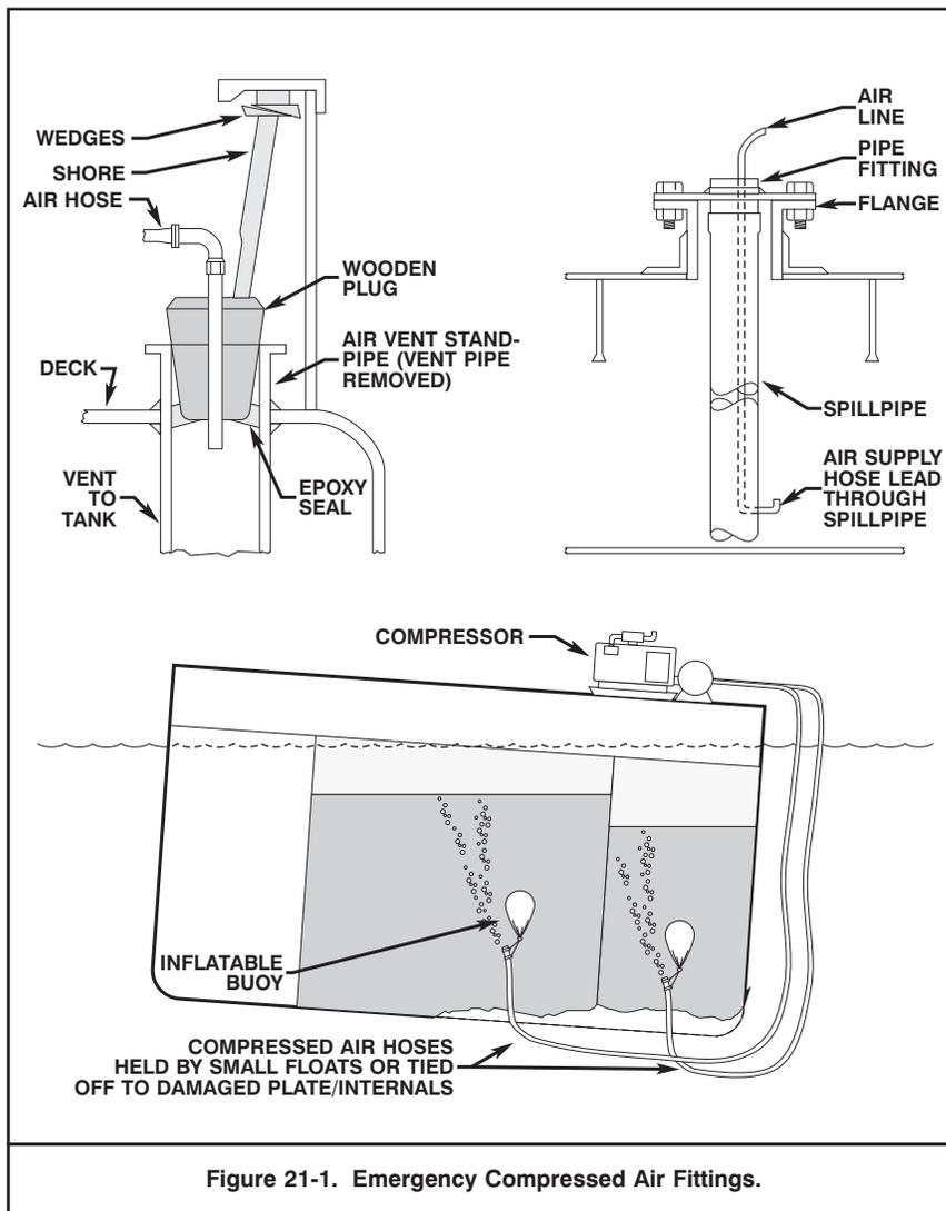
Figure 21-1. Emergency Compressed Air Fittings.
