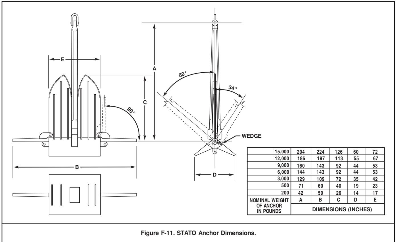
Figure F-11. STATO Anchor Dimensions.
