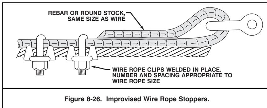
Figure 8-26. Improved Wire Rope Stoppers.
