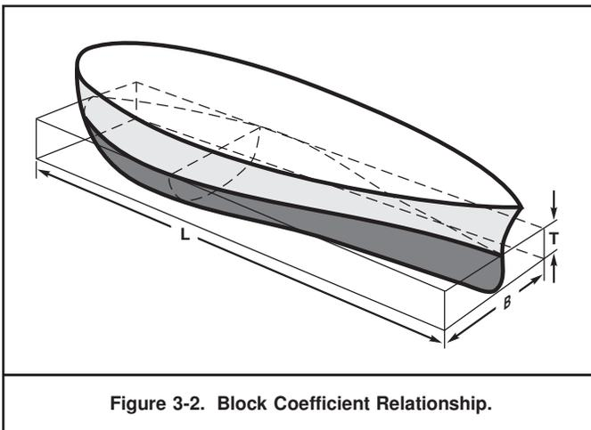
Figure 3-2. Block Coefficient Relationship.
