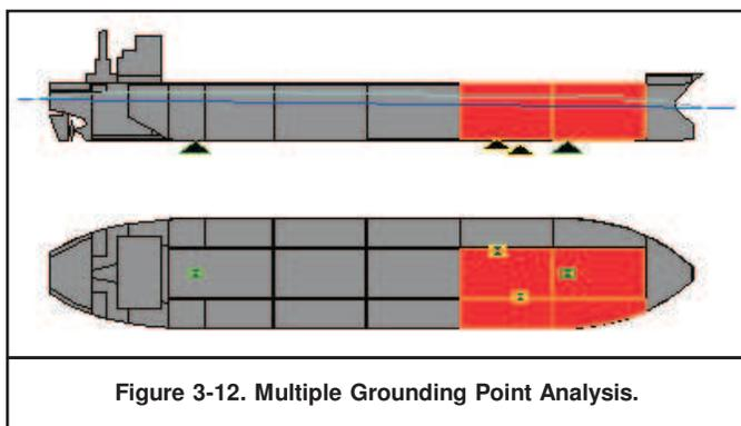
Figure 3-12. Multiple Grounding Point Analysis.
