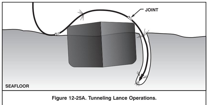
Figure 12-25A. Tunneling Lance Operations.
