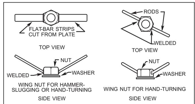
Figure 10-34. Wing Nuts for Salvage Patches.
