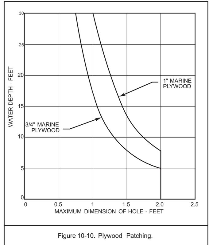
Figure 10-10. Plywood Patching.
