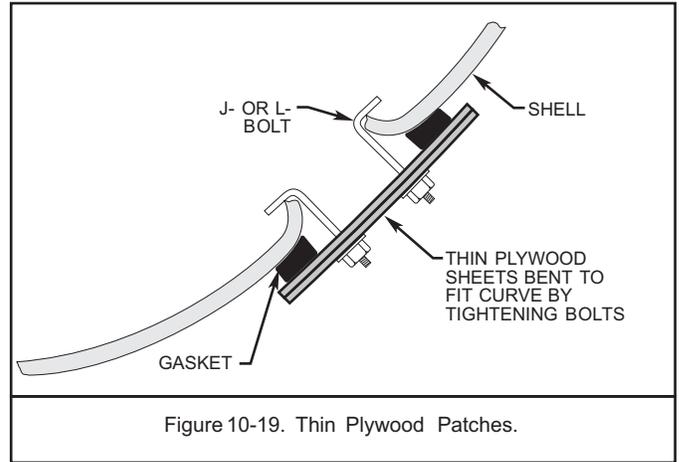
Figure 10-19. Thin Plywood Patches.
