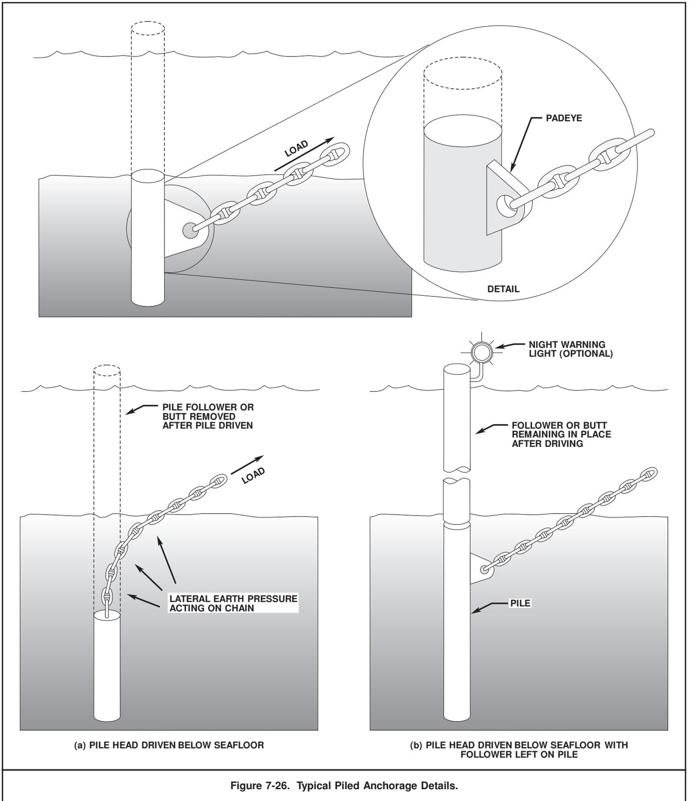
Figure 7-26. Typical Piled Anchorage Details.
