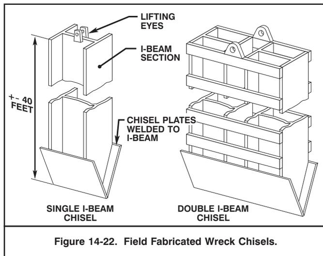
Figure 14-22. Field Fabricated Wreck Chisels.
