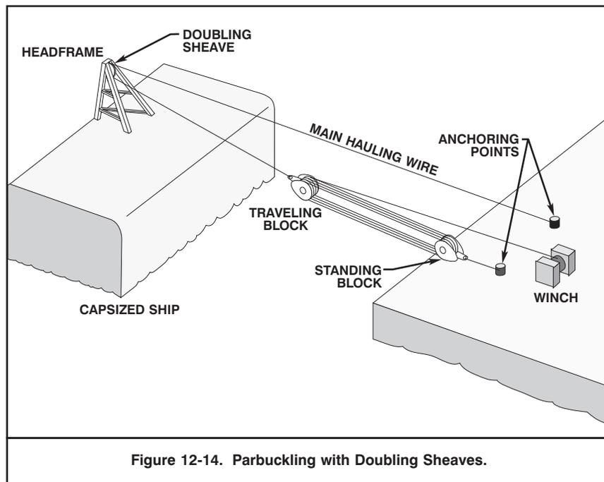
Figure 12-14. Parbuckling with Doubling Sheaves.
