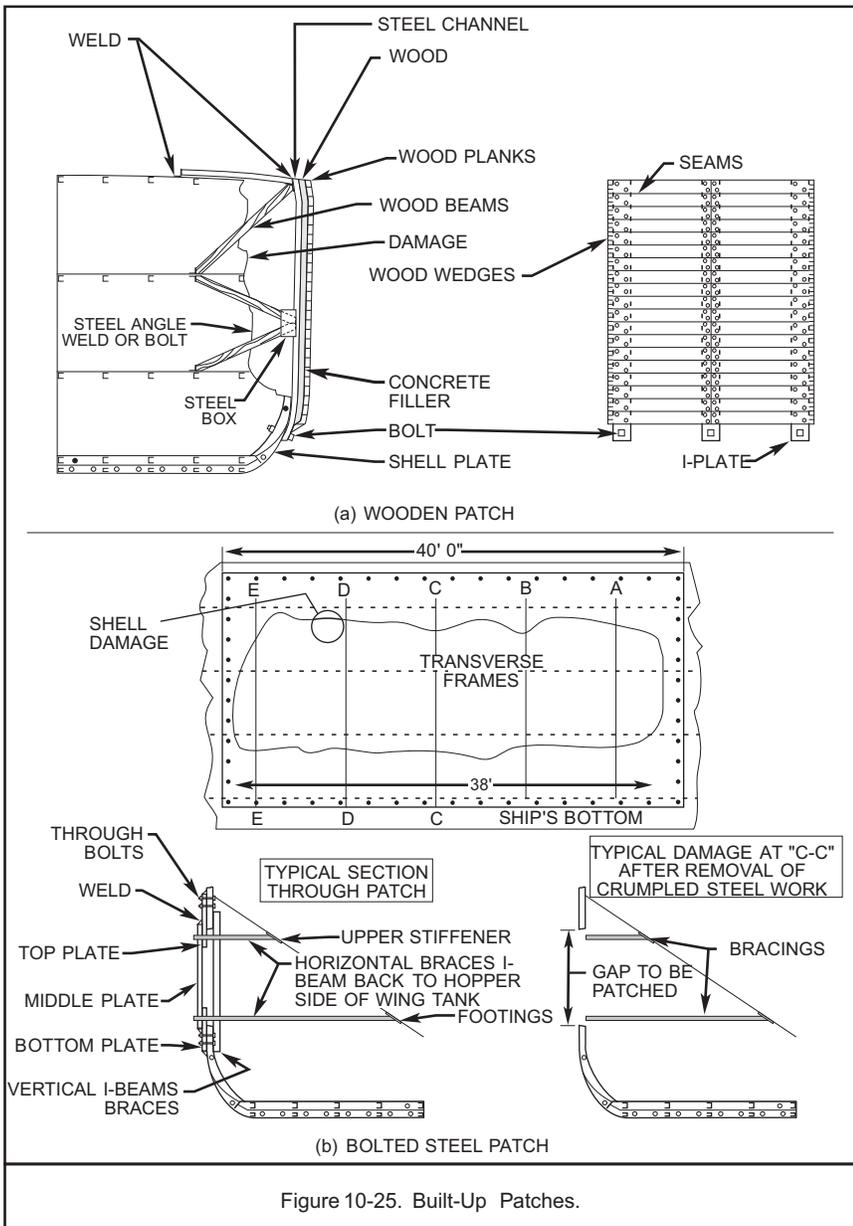
Figure 10-25. Built-Up Patches.
