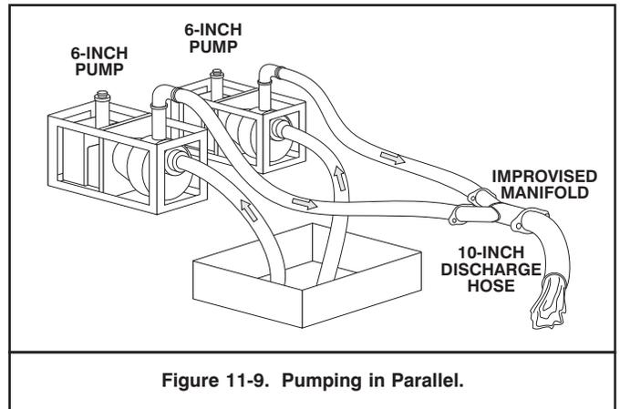
Figure 11-9. Pumping in Parallel.
