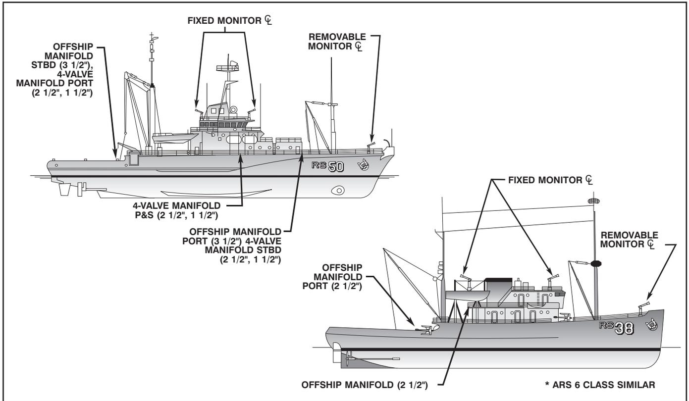
Figure 17-2A. Salvage Ship Offship Firefighting Systems.
