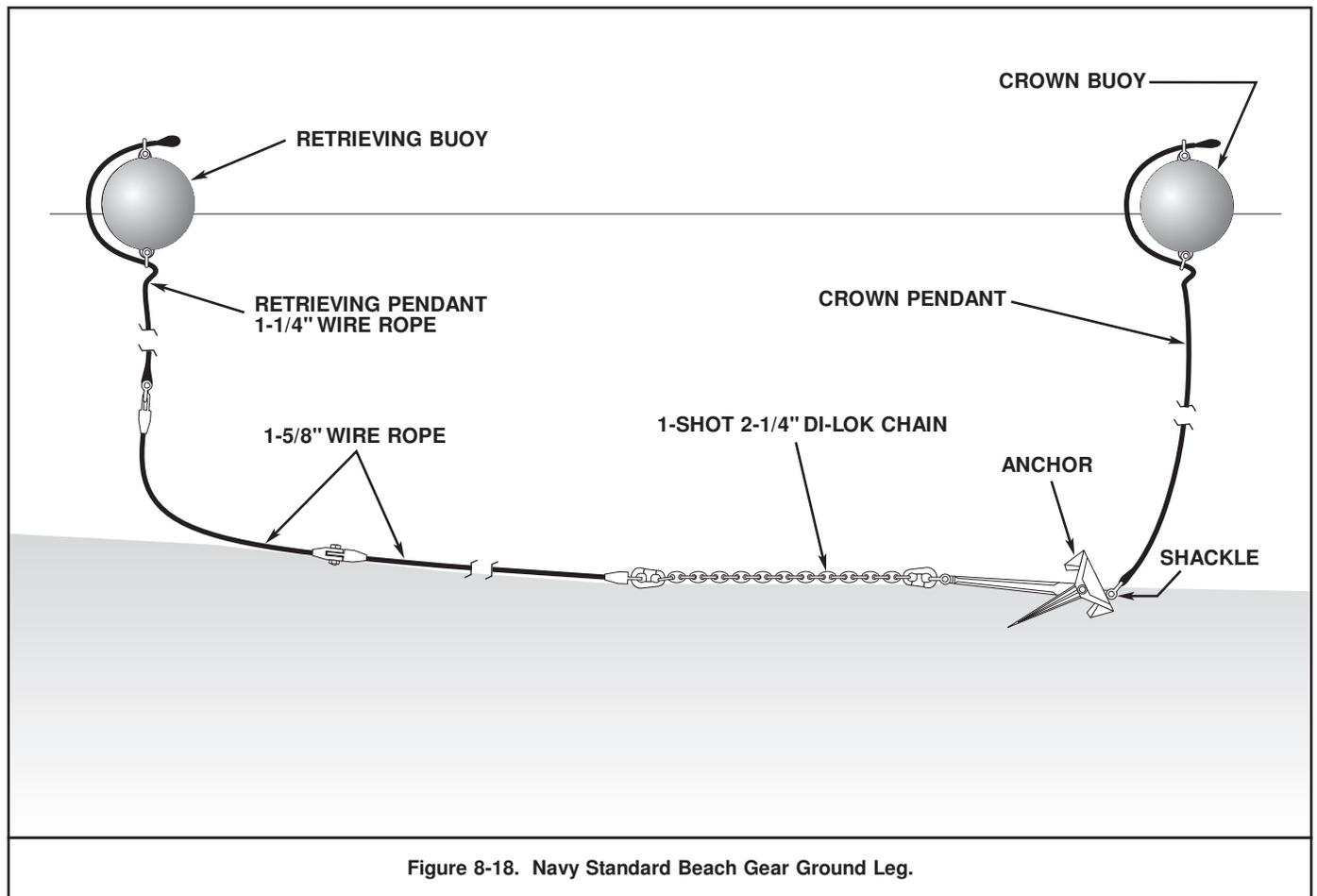
**Figure 8-18. Navy Standard Beach Gear Ground Leg.**
