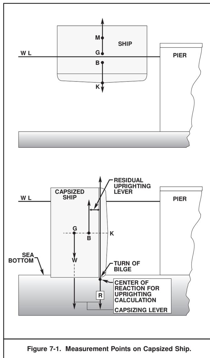
Figure 7-1. Measurement Points on Capsized Ship.
