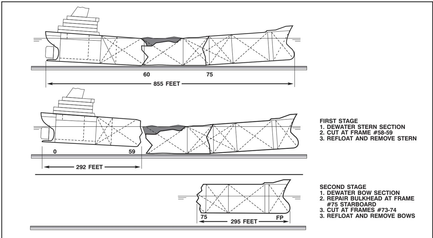
Figure 14-5. Removal of Bow and Stern Sections of Wreck.
