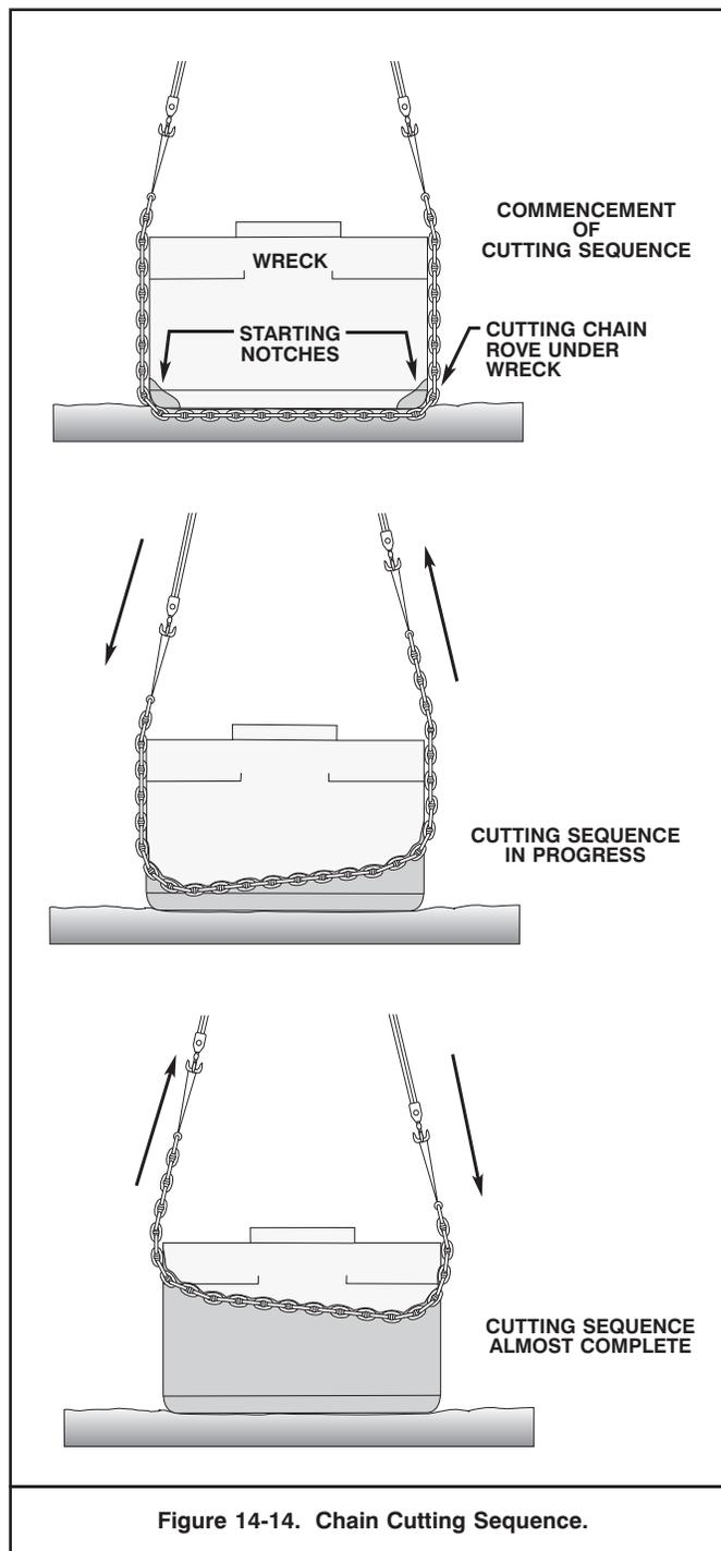
Figure 14-14. Chain Cutting Sequence.
