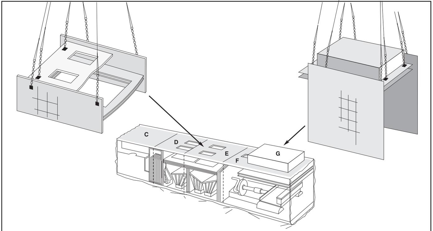
Figure 14-8. Status of a Wreck Before Horizontal Cuts Commence.
