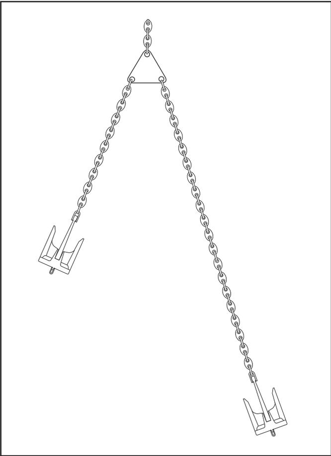
Figure 8-11. Doubled Anchor Arrangement.
