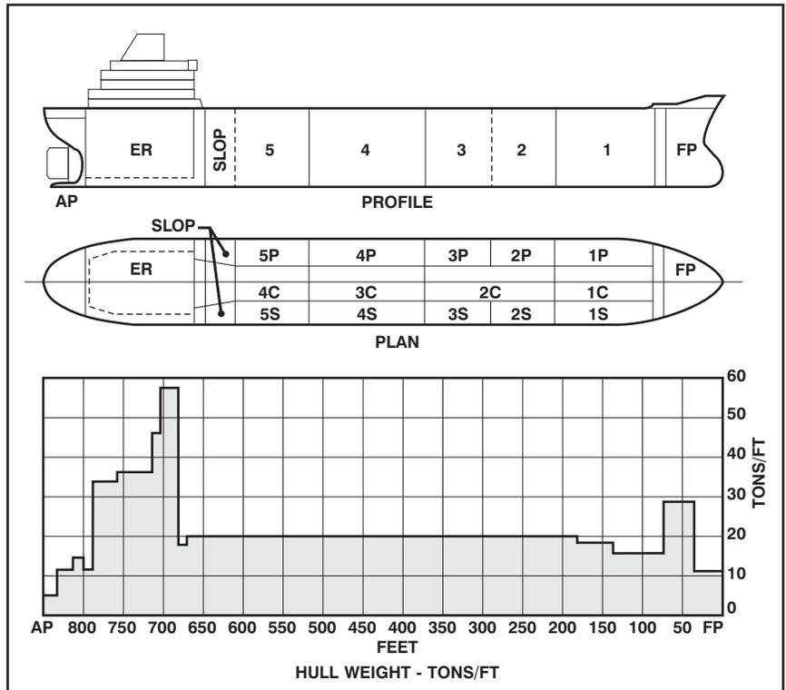
Figure 14-3. Weight Distribution Curve for a Large Tanker.
