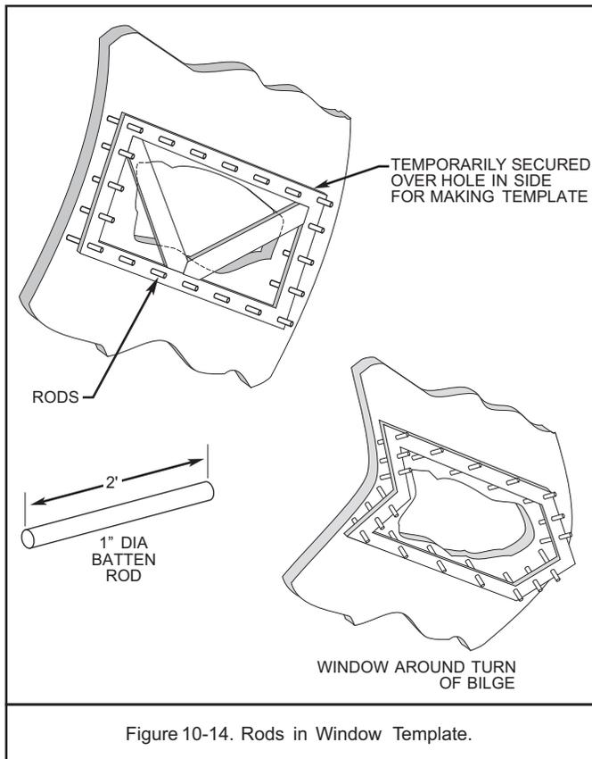
Figure 10-14. Rods in Window Template.
