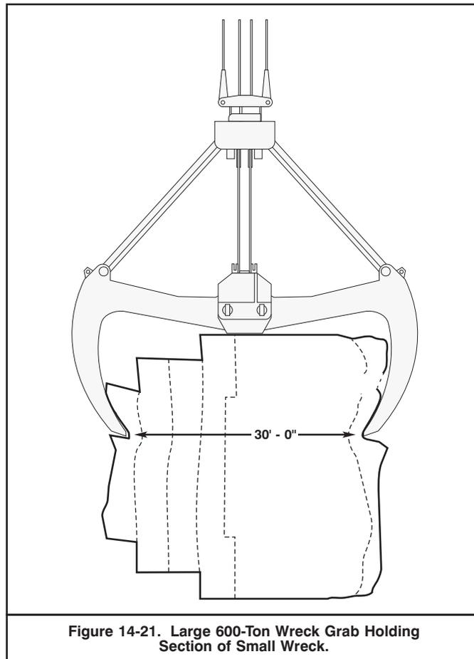
**Figure 14-21. Large 600-Ton Wreck Grab Holding Section of Small Wreck.**
