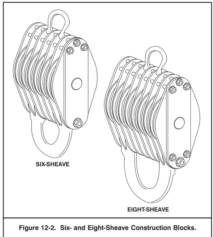
Figure 12-2. Six- and Eight-Sheave Construction Blocks.
