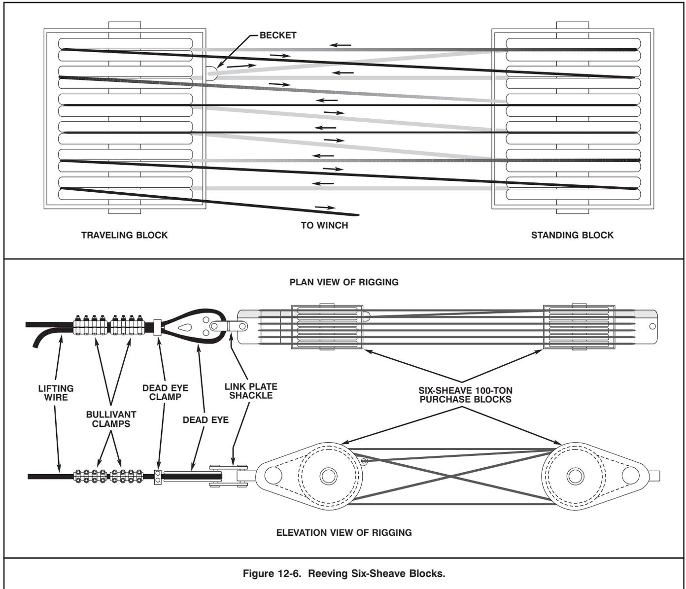
Figure 12-6. Reeving Six-Sheave Blocks.
