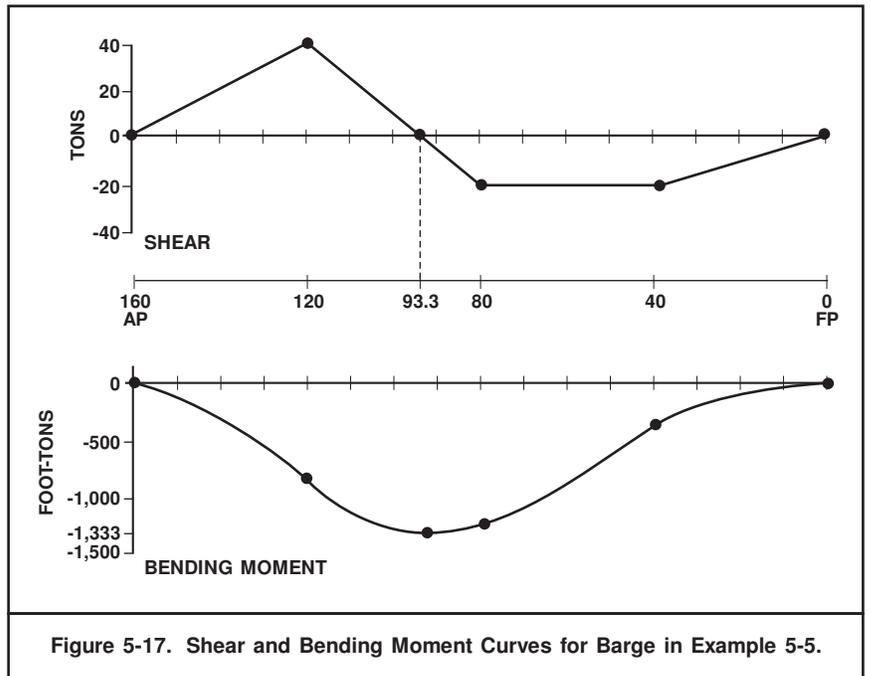
Figure 5-17. Shear and Bending Moment Curves for Barge in Example 5-5.
