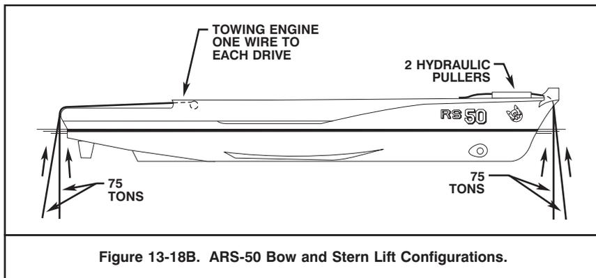
Figure 13-18B. ARS-50 Bow and Stern Lift Configurations.
