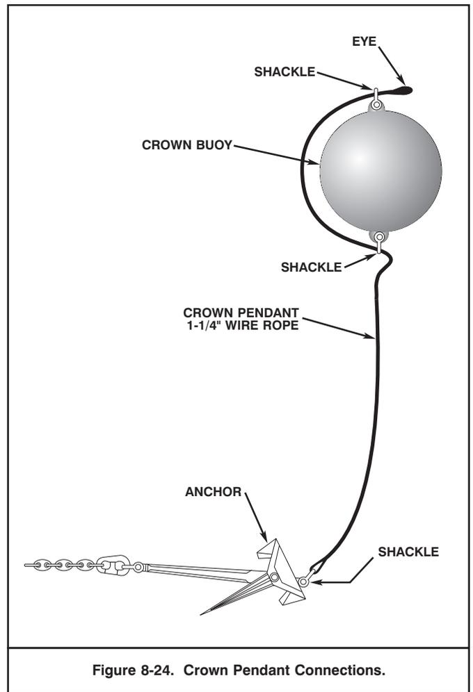
Figure 8-24. Crown Pendant Connections.
