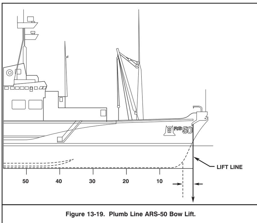
Figure 13-19. Plumb Line ARS-50 Bow Lift.
