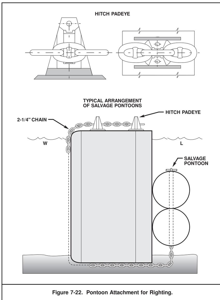
Figure 7-22. Pontoon Attachment for Righting.
