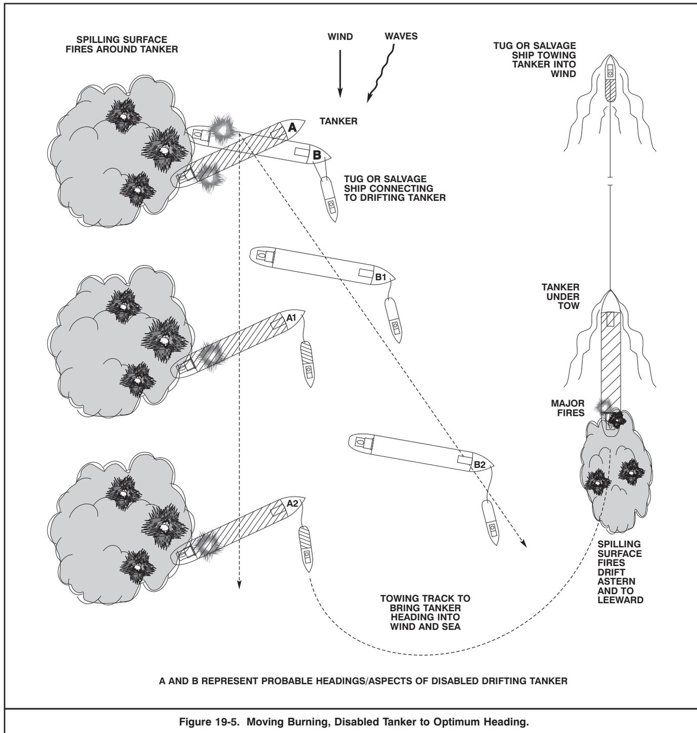
Figure 19-5. Moving Burning, Disabled Tanker to Optimum Heading.
