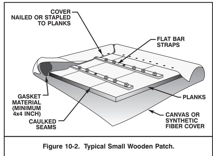
Figure 10-2. Typical Small Wooden Patch.
