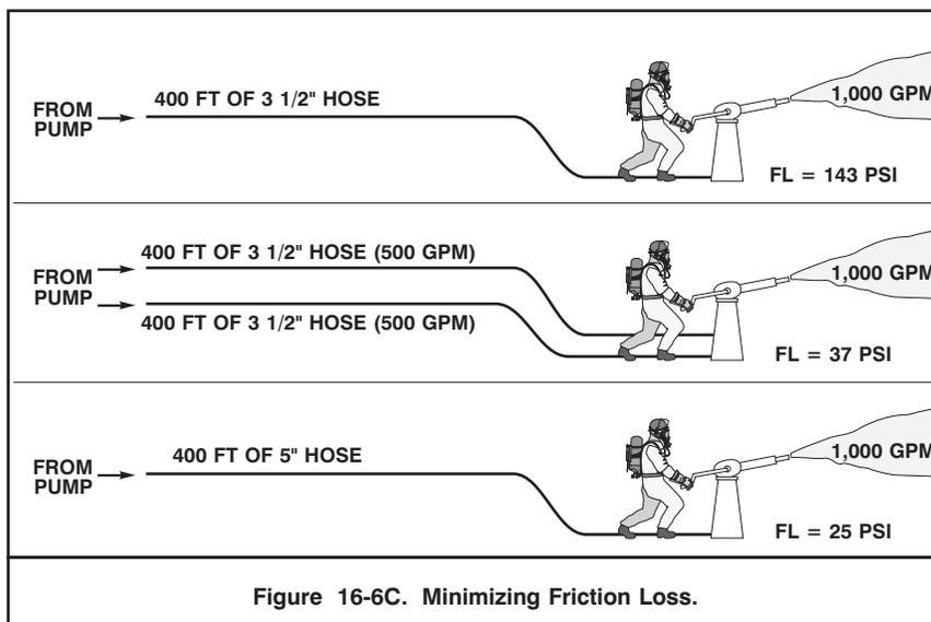
Figure 16-6C. Minimizing Friction Loss.
