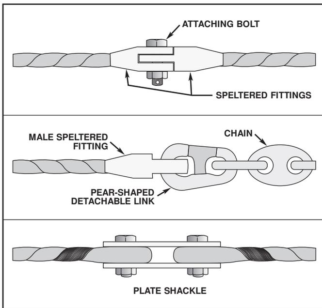
Figure 8-21. Connections for Ground Leg.
