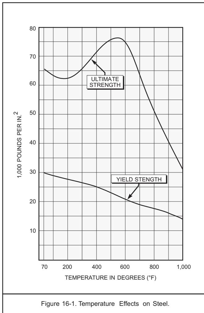
Figure 16-1. Temperature Effects on Steel.
