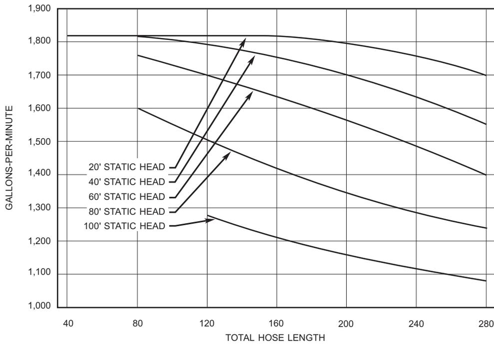
Figure H-11. CCN-150 Flow Rates - Water, 6" Hose.
