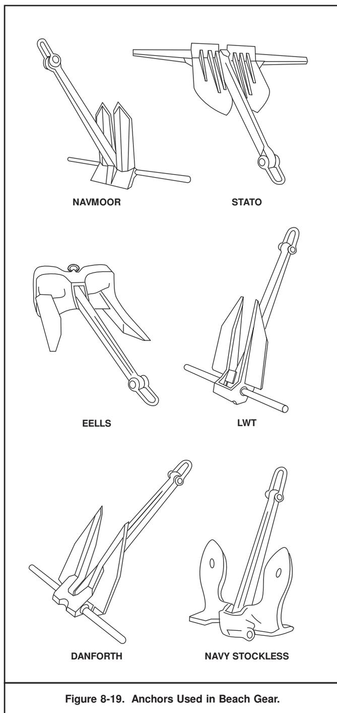
Figure 8-19. Anchors Used in Beach Gear.
