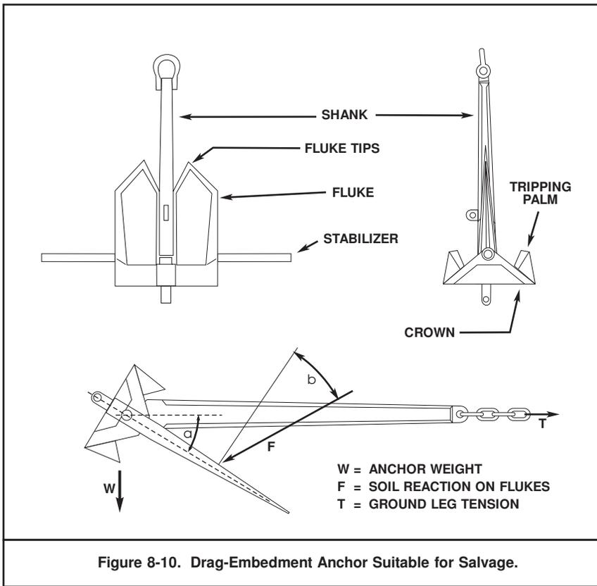
Drag-embedment anchors are manufactured in a wide variety of sizes and shapes, but all have common characteristics. As shown in Figure 8-10, drag-embedment anchors suitable for salvage are made up of the following parts:
