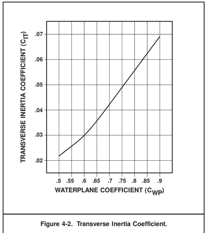
Figure 4-2. Transverse Inertia Coefficient.
