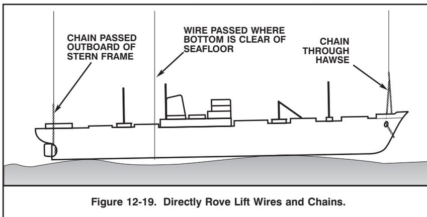
Cranes, bridges, and other sunken structures often encountered in harbor clearance operations are frequently directly rove. The open lattice and chord construction, and the inherent strength of crane and bridge sections, make them especially suitable for this method.
