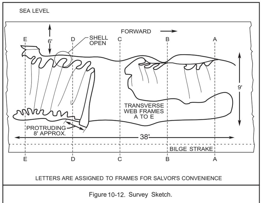
The survey does not produce an engineering specification for a salvage patch, although it does produce adequate information and measurements for the salvage engineer to calculate the strength of the patch and proceed with an initial design.
