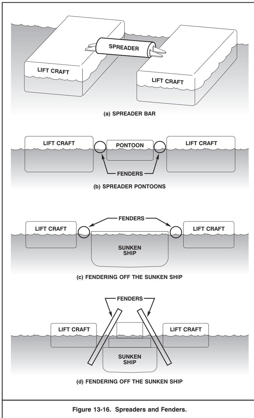
Figure 13-16. Spreader Bars and Fenders.
