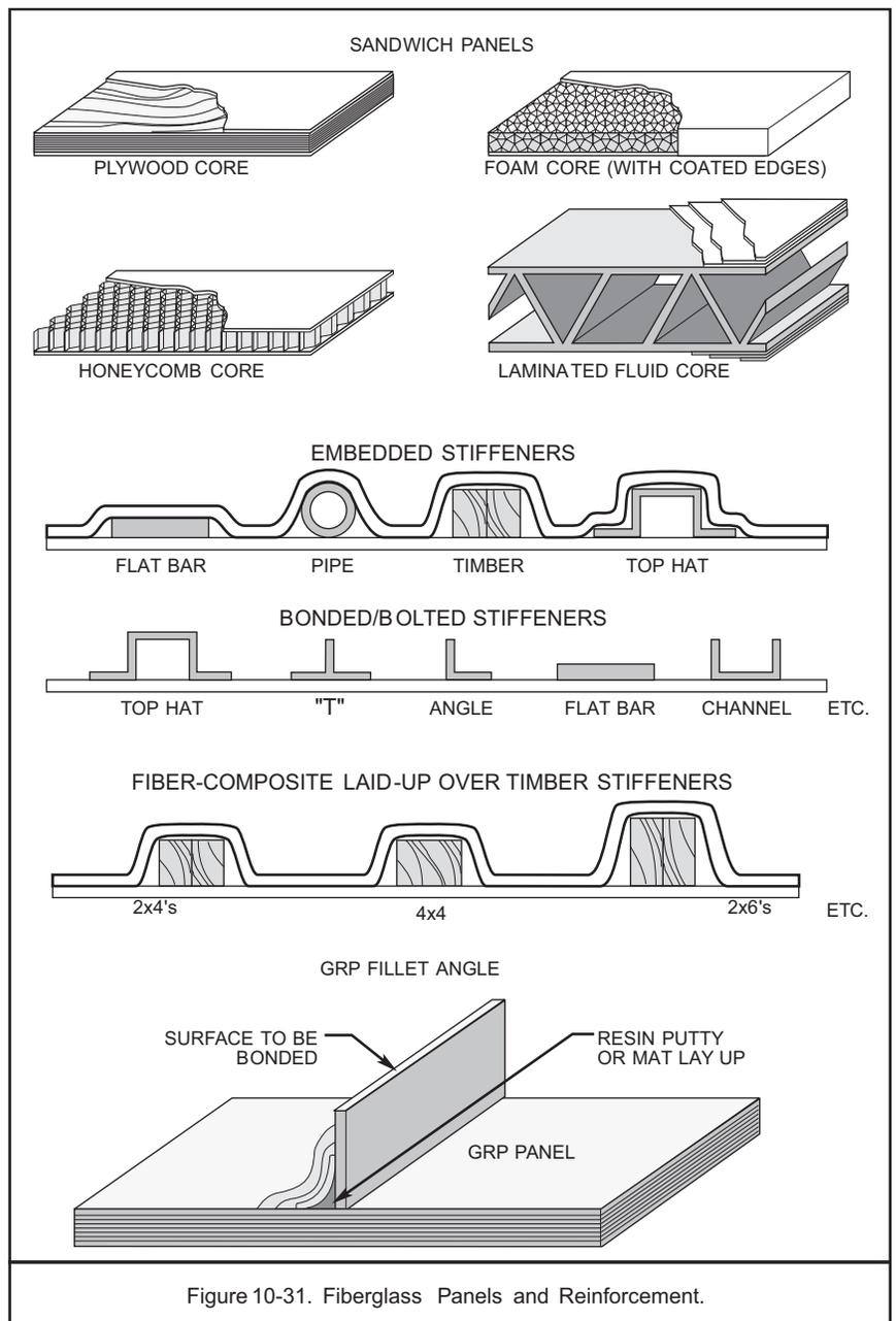
Figure 10-31. Fiberglass Panels and Reinforcement.
