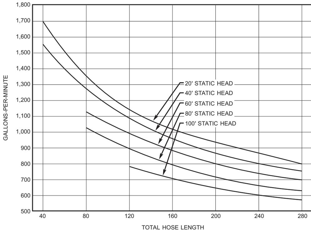
Figure H-10. CCN-150 Flow Rates - Water, 4" Hose.
