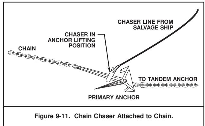
Figure 9-11. Chain Chaser Attached to Chain.
