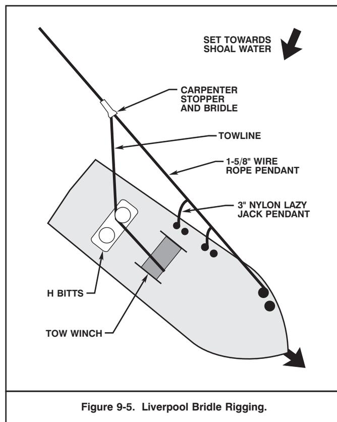
Figure 9-5. Liverpool Bridle Rigging.
