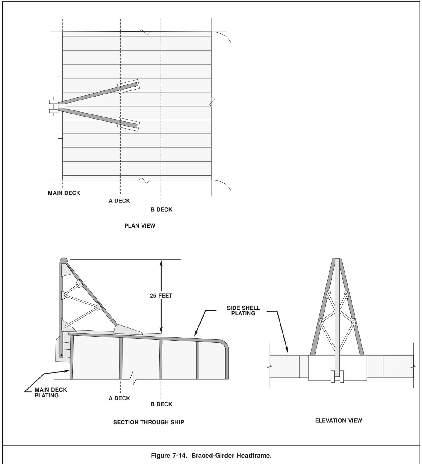
Figure 7-14. Braced-Girder Headframe.
