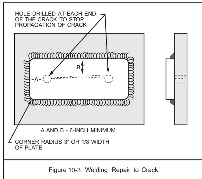
Figure 10-3. Welding Repair to Crack.
