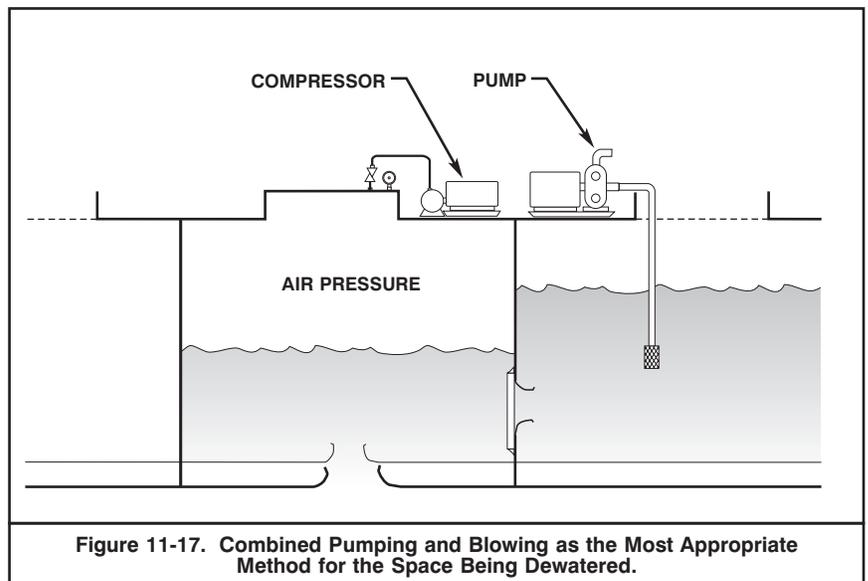
Combined pumping and blowing operations are tedious and must be undertaken only with a full appreciation of the problems involved in situations where they are clearly called for and the alternatives are unacceptable.
