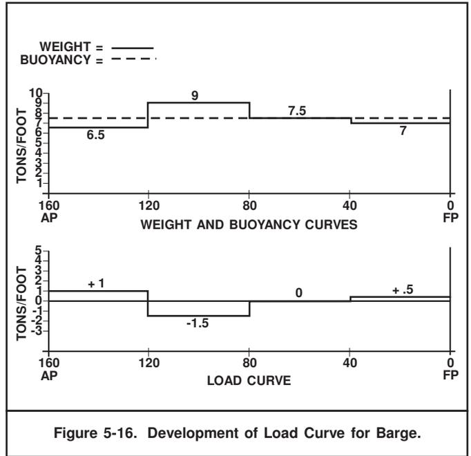
Figure 5-16. Development of Load Curve for Barge.
