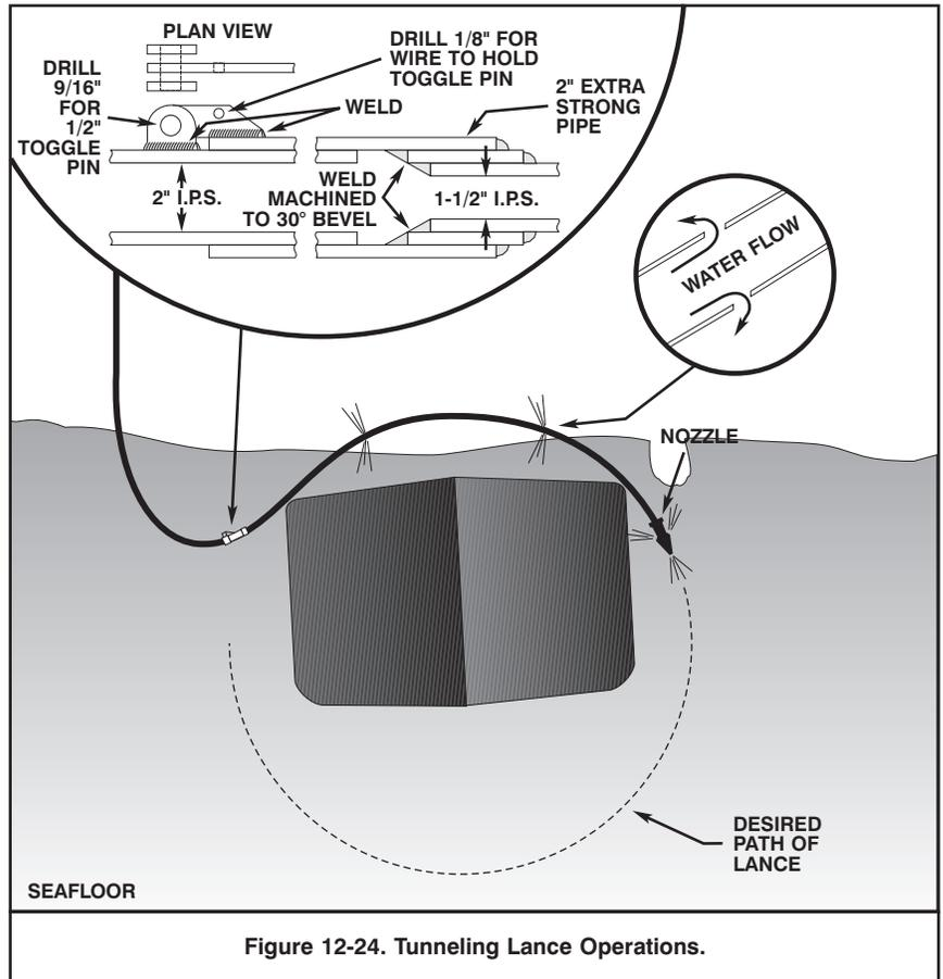
Figure 12-24. Tunneling Lance Operations.
