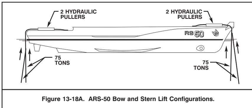
Figure 13-18A. ARS-50 Bow and Stern Lift Configurations.
