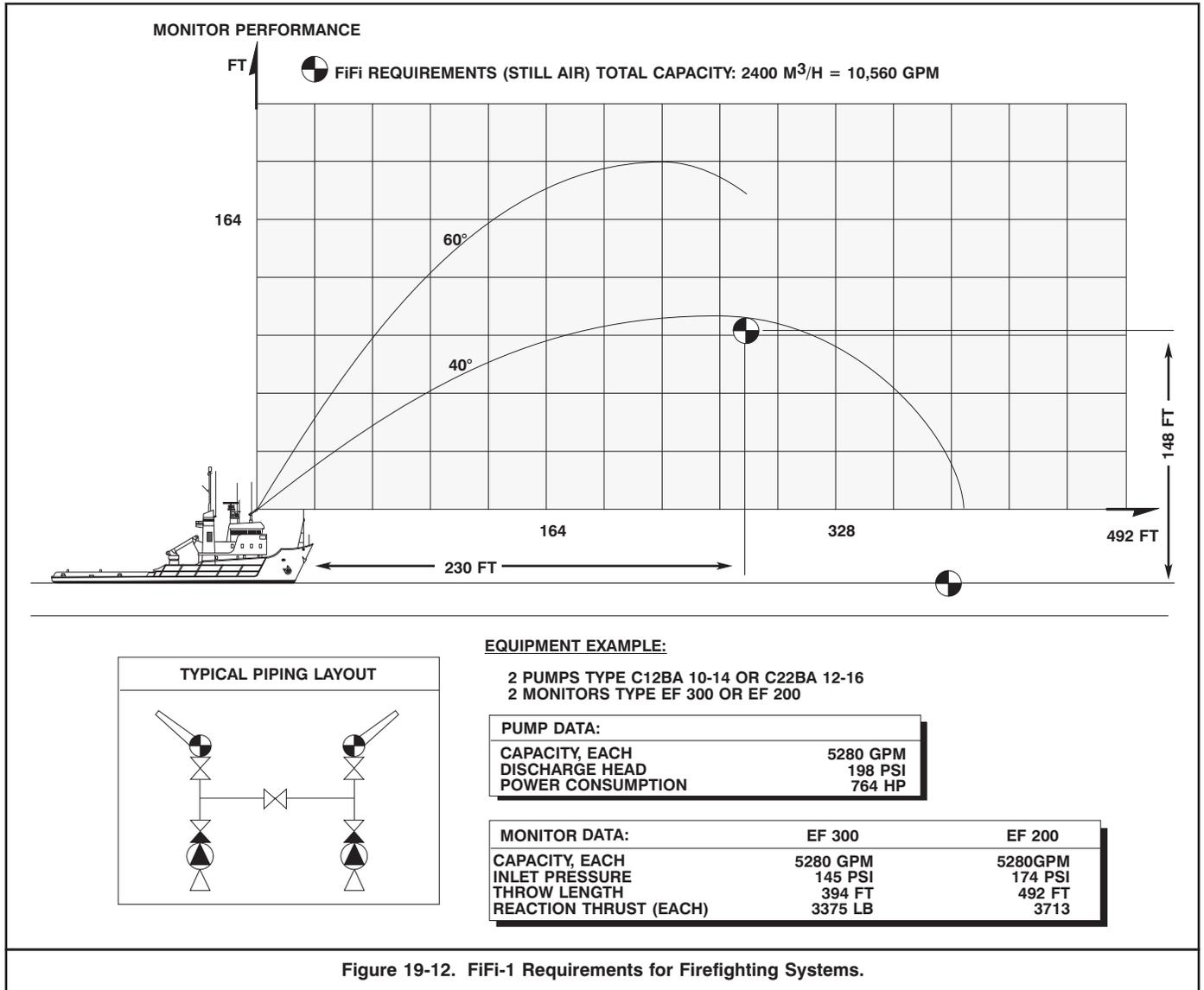
Figure 19-12. FiFi-1 Requirements for Firefighting Systems.
