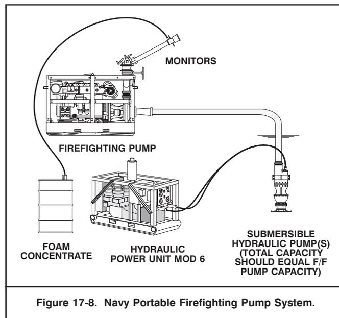
Figure 17-8. Navy Portable Firefighting Pump System.
