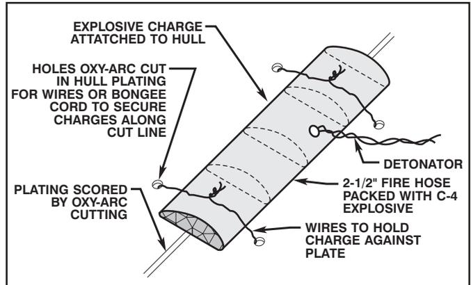
Figure 14-25. Hose-Type Cutting Charge.
