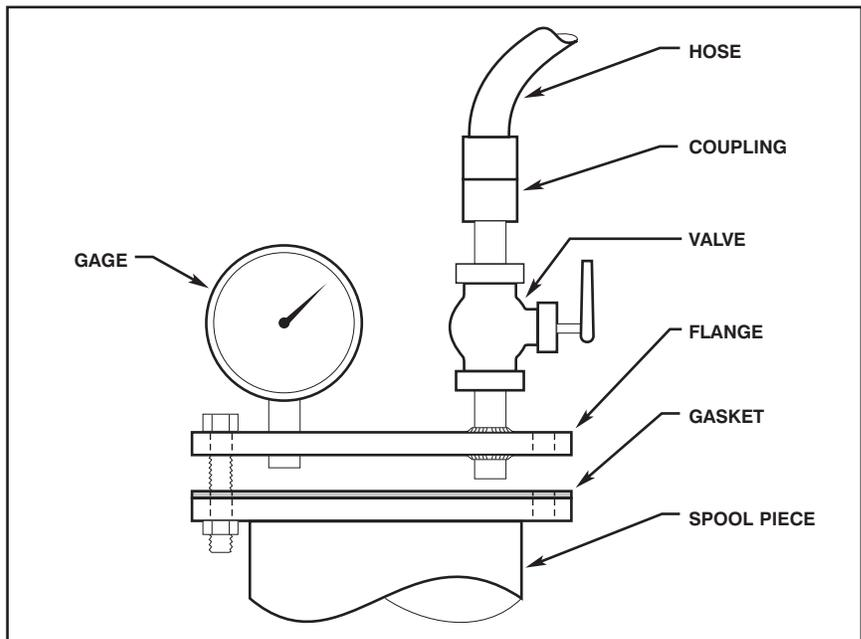
Figure 11-12. Blowing Fitting.
