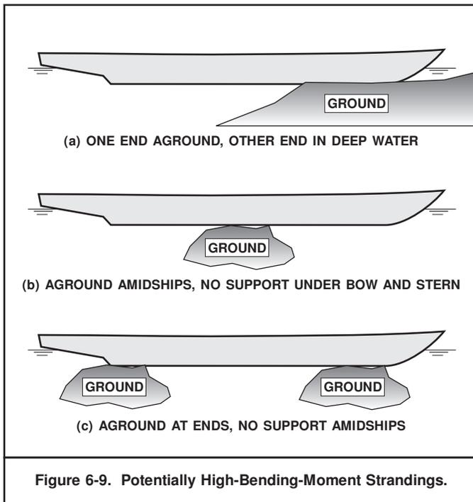
Figure 6-9. Potentially High-Bending-Moment Strandings.
