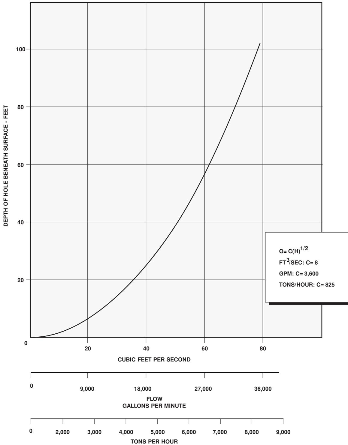
Figure 6-8. Flow Through a One-Square-Foot Hole.
