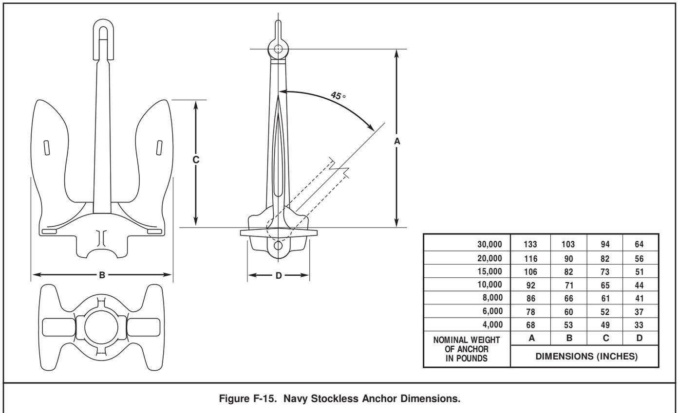
Figure F-15. Navy Stockless Anchor Dimensions.
