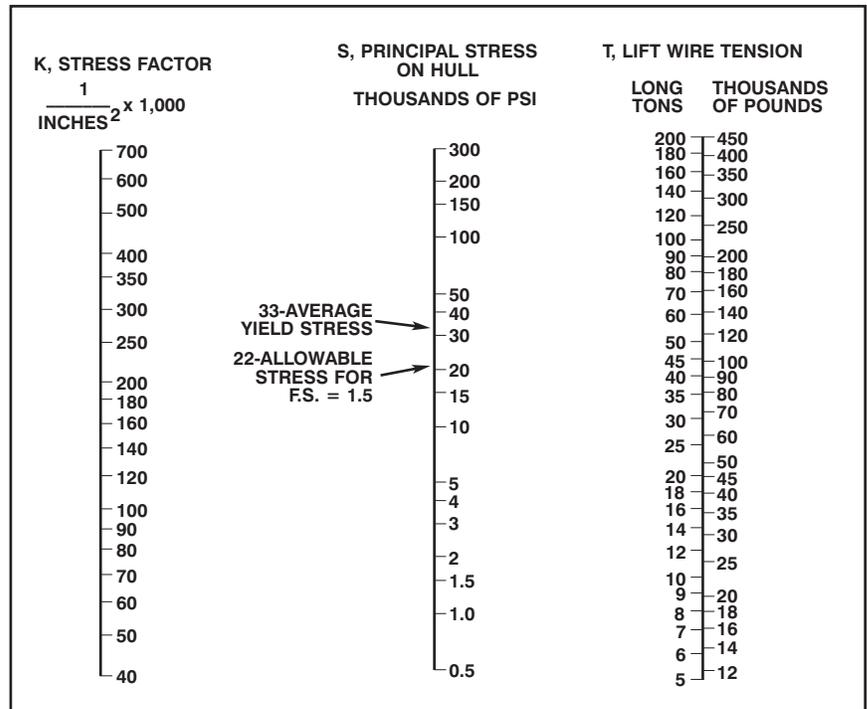
**Figure 12-17. Hull Stress Nomogram.**
