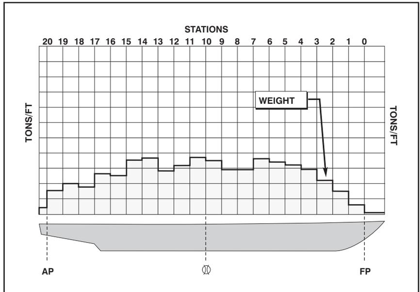
Figure 14-2. Weight Curve for Frigate.
