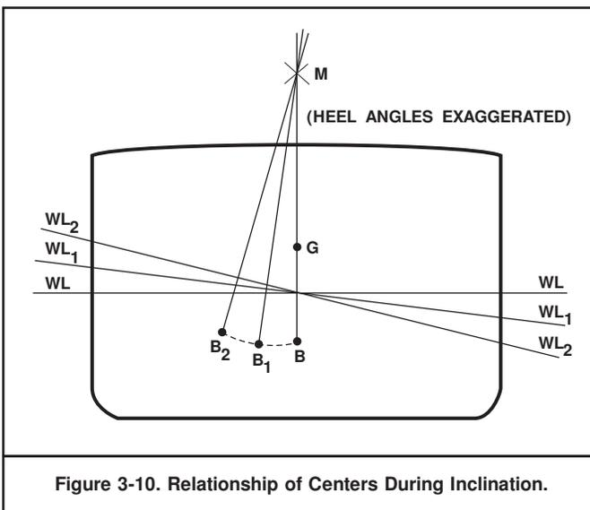
Figure 3-10. Relationship of Centers During Inclination.
