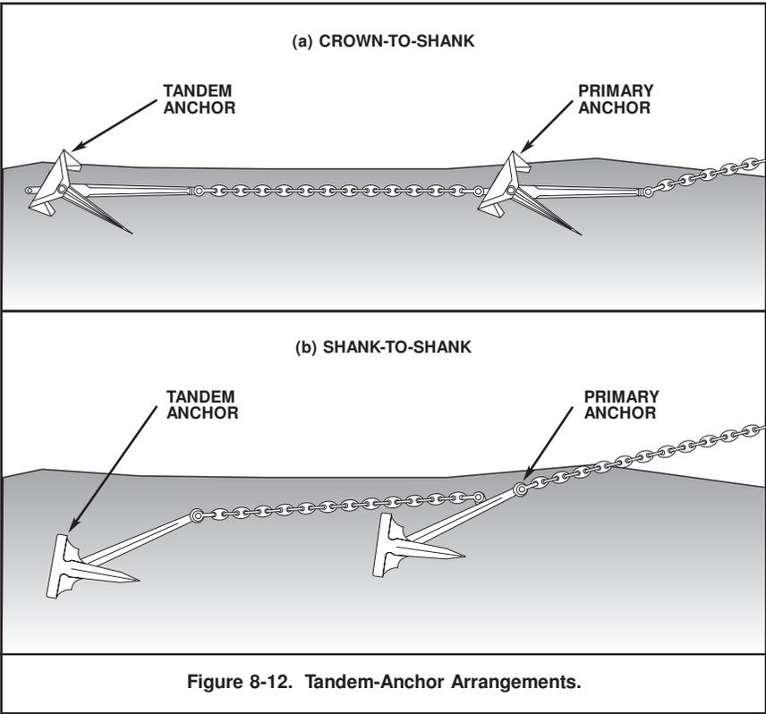
Figure 8-12. Tandem-Anchor Arrangements.
