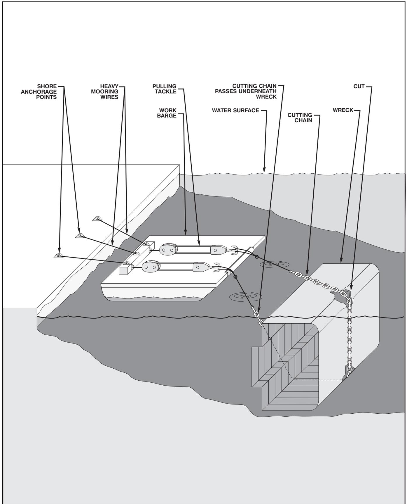
Figure 14-18. Horizontal Chain Cutting System.
