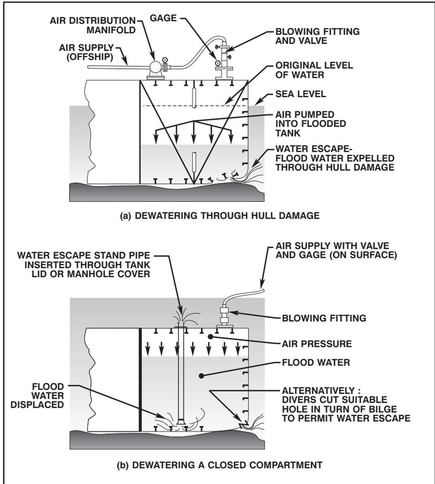
Figure 11-11. Compressed Air System.
