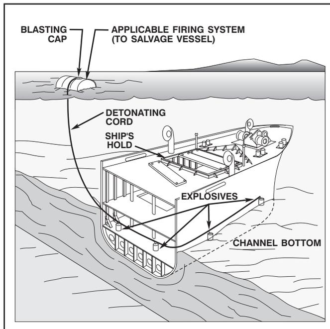
Figure 14-29. Charge Placement for Wreck Settling.
