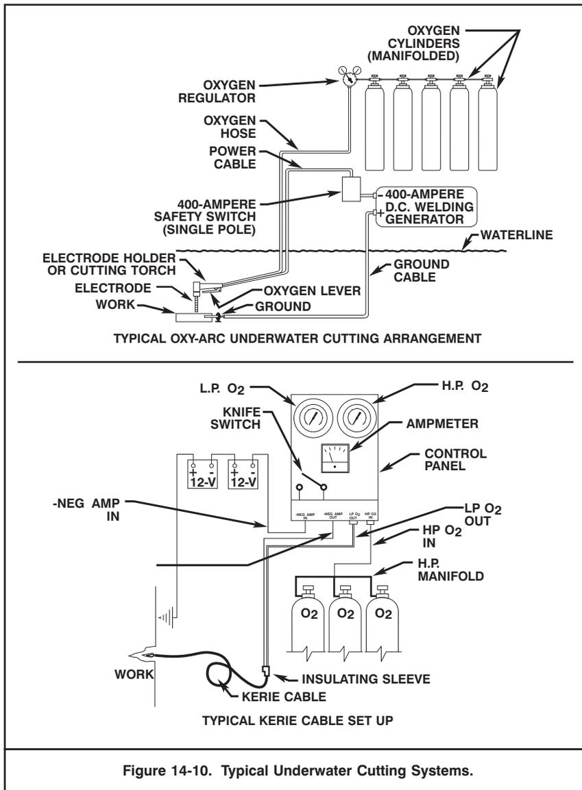
Figure 14-10. Typical Underwater Cutting Systems.
