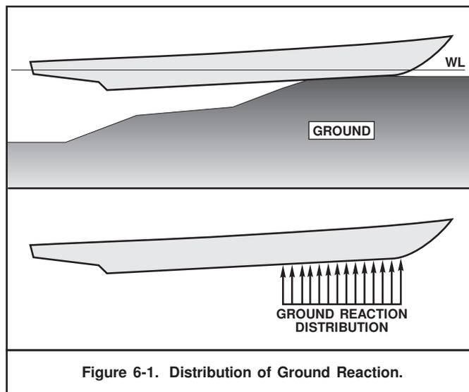
Figure 6-1. Distribution of Ground Reaction.
