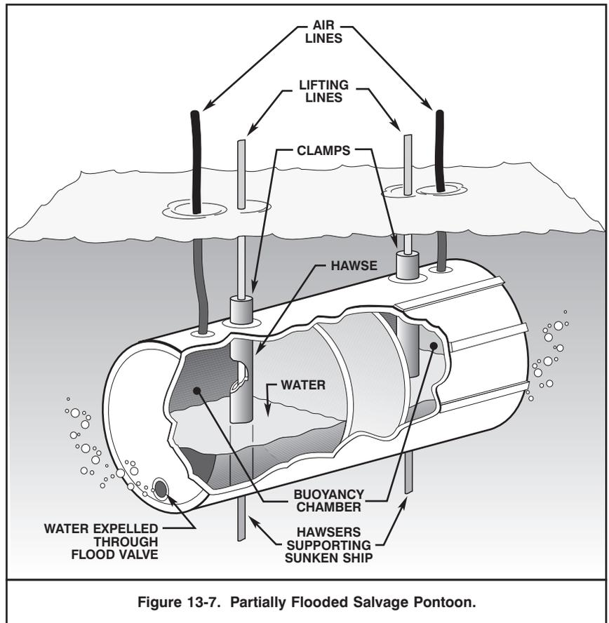
Figure 13-7. Partially Flooded Salvage Pontoon.
