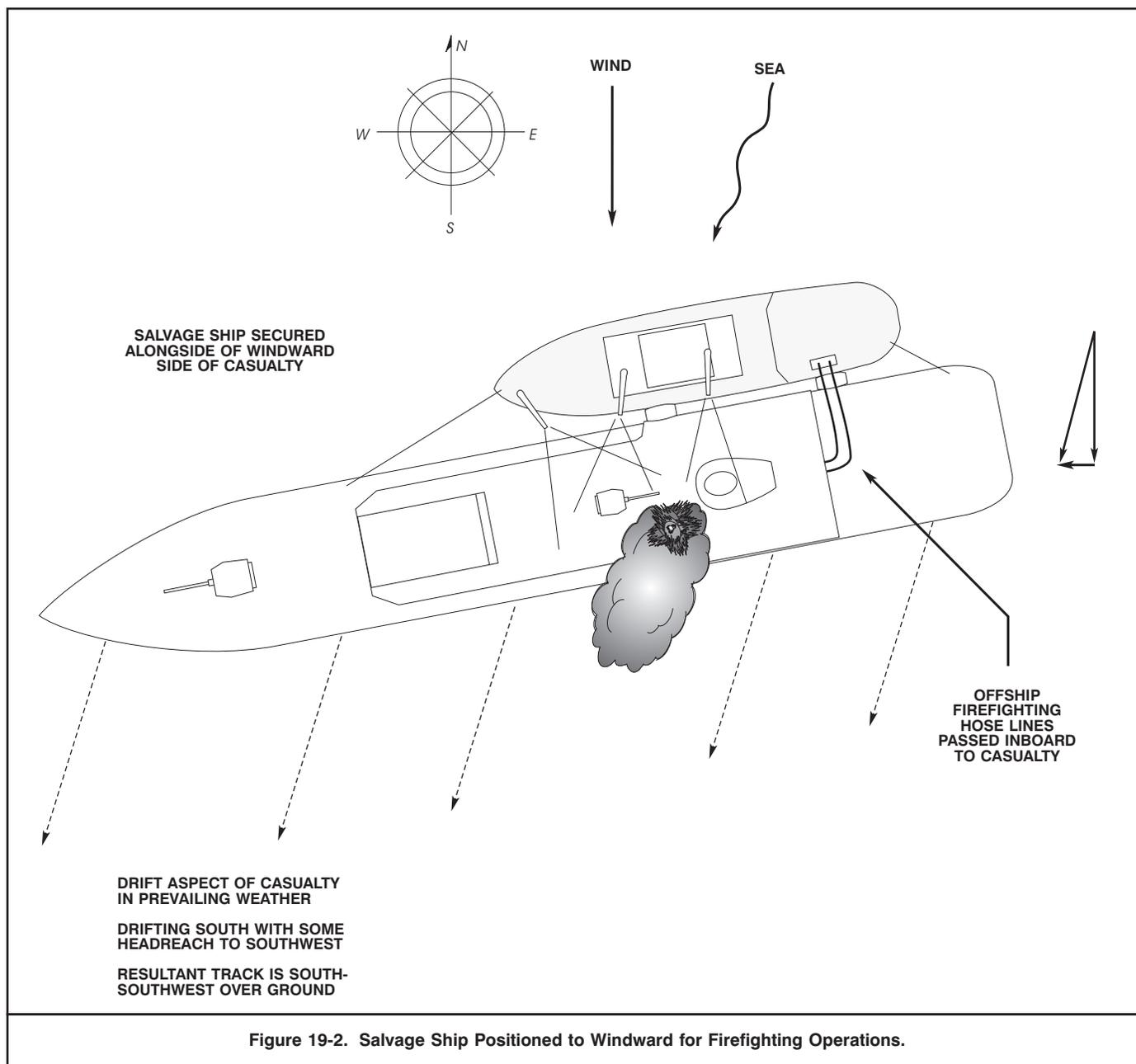
**Figure 19-2. Salvage Ship Positioned to Windward for Firefighting Operations.**
