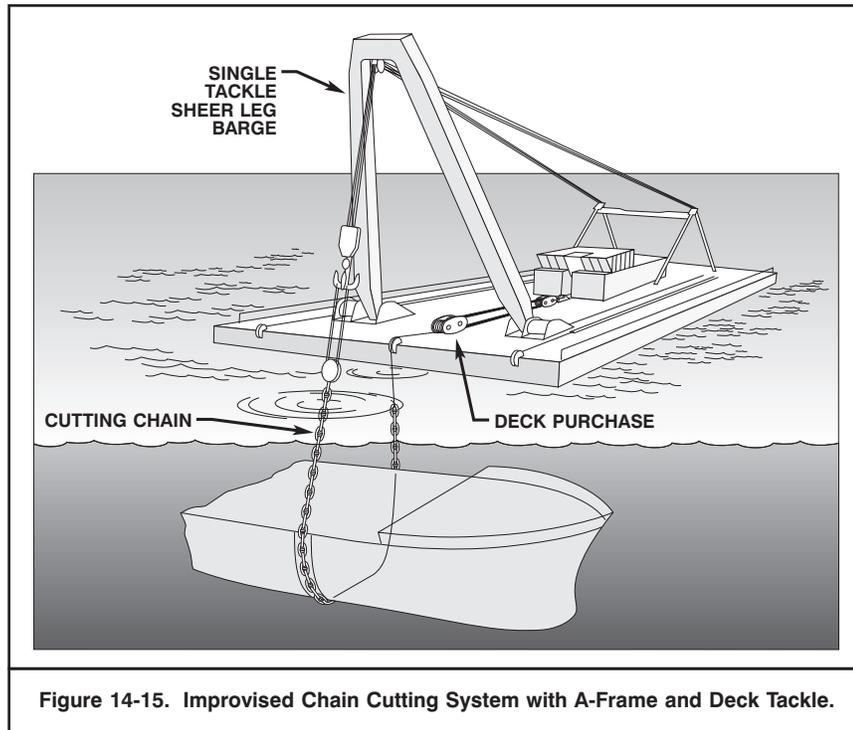
Figure 14-15. Improvised Chain Cutting System with A-Frame and Deck Tackle.
