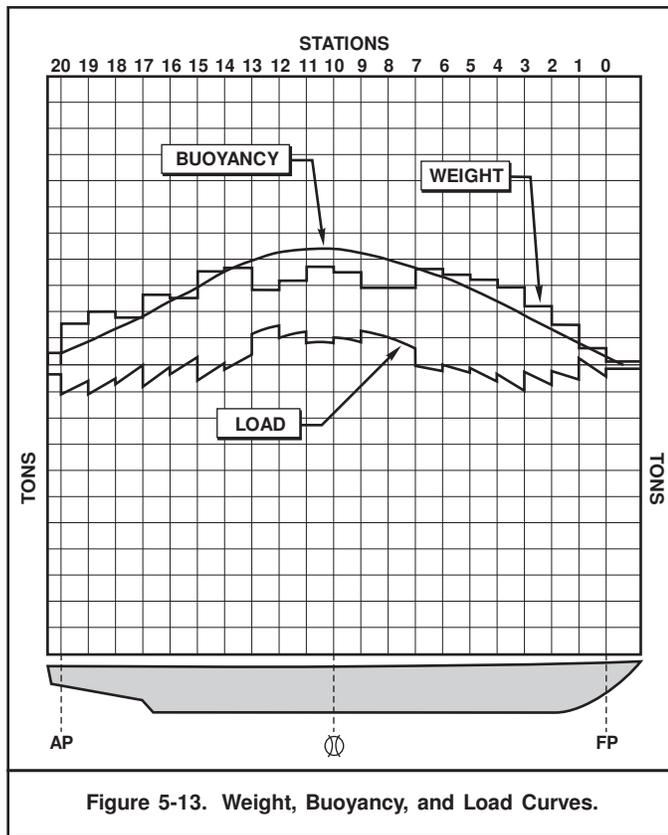
Figure 5-13. Weight, Buoyancy, and Load Curves.
