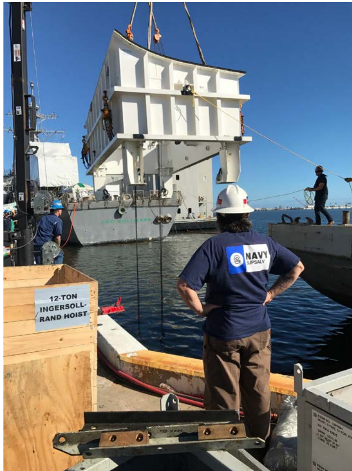
Upper section of the cofferdam being lowered into the water in preparation to begin port side rudder repairs. Note the stern of THE SULLIVANS in the background and NAVSEA UWSH Operations Specialist, Russ Mallet monitoring.
