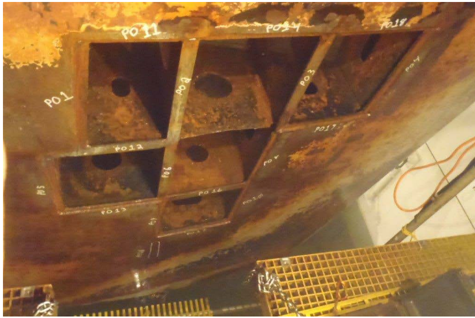
A view of the port rudder with shell plating removed during weld repairs.
