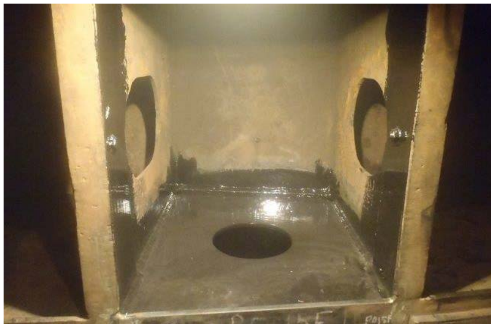
Interior of a rudder void after weld repairs and preservation.
