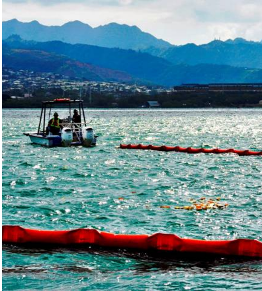
25' Utility boat herding yellow wooden blocks, simulating spilled product, during training maneuvers.
