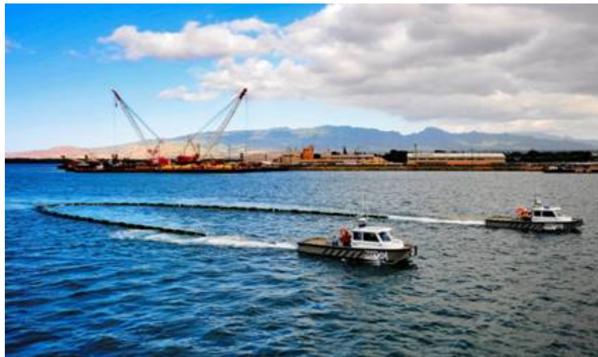
Two 30' Boom Handling Boats performing half-moon skimming maneuver.
