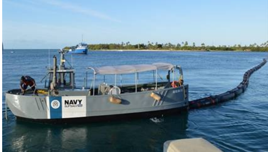
Class V Modular Vessel Skimmer getting underway from Alpha 7 pier in Pearl Harbor Naval Base. This skimmer system uses an absorbent belt to collect oil product herded by its booms.
