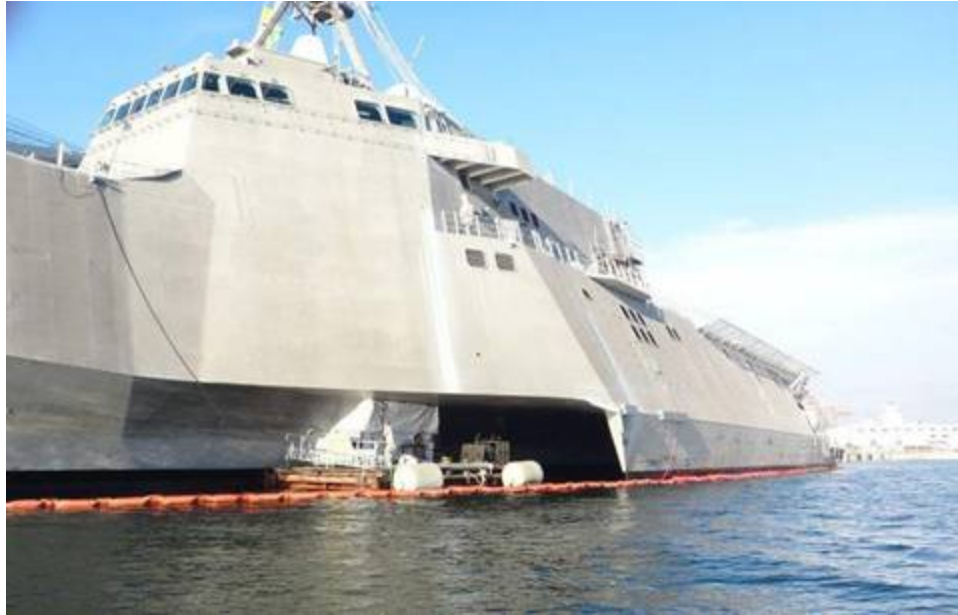
USS INDEPENDENCE (LCS 2) pier side with welding barge positioned for Hull Mounting Plate installation.
