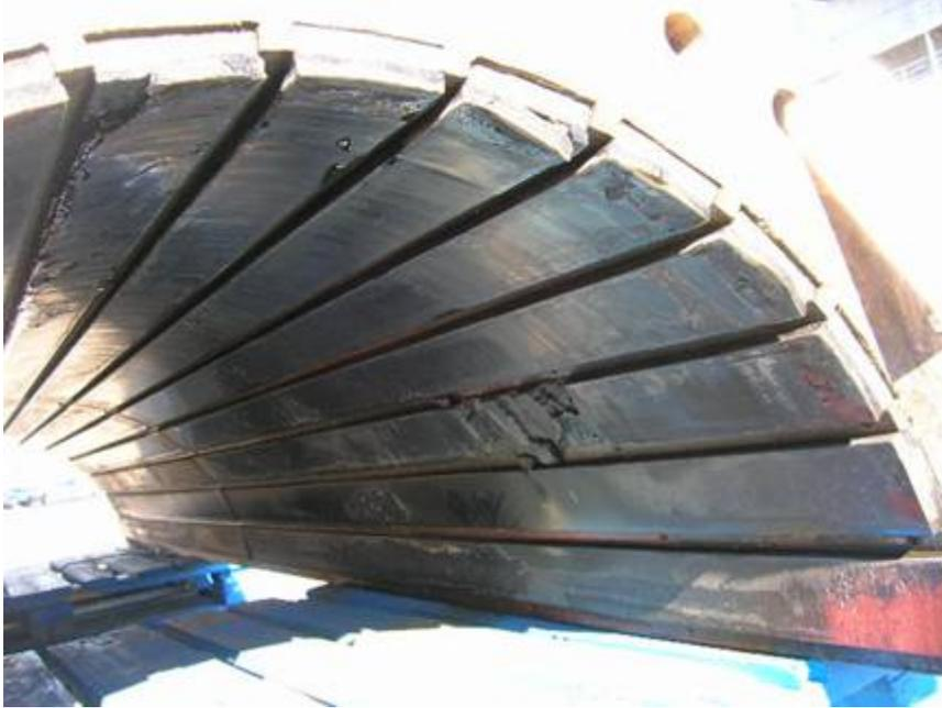
This image shows damage to the lower half of IKE's number 3 shaft bearing. After rigging the damaged bearing ashore, a Norfolk Naval Shipyard machine shop will remove all the old staves and re-install new ones. SUPSALV will then rig them back under the ship for installation. It is anticipated the entire task will take between 4 and 5 weeks to accomplish.
