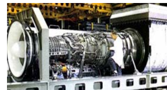
LM-2500 Propulsion System
