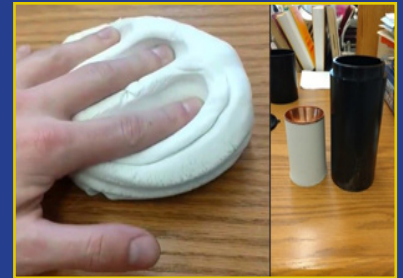
Left: FPEX demonstrating pliability characteristics Right: FPEX packed and formed into a shape charge
