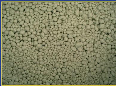
SEM Image of Tungsten Delay Composition, 1x20 Magnification
