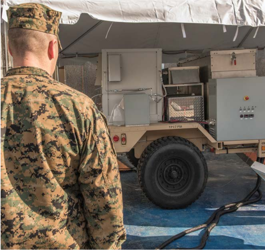
Lt. Col. William P. Dobbins, an engineer for U.S. Marine Corps Forces Command, watches a demonstration and test kickoff of the first logistics fuel (JP-8) compatible renewable-hybrid Solid Oxide Fuel Cell (SOFC) system Jan. 26, 2017, at Naval Surface Warfare Center, Carderock Division in West Bethesda, Md. (U.S. Navy photo by Jacob Cirkse/Released)
