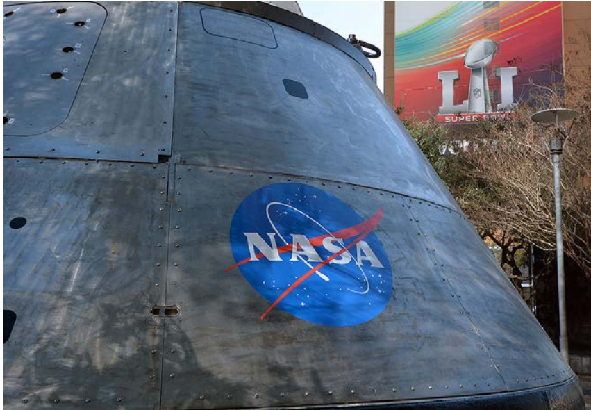
NASA's Post-landing Orion Recovery Tests (PORT) capsule is seen on display at the Super Bowl LIVE festival in Houston. The full-scale model, weighing 18,000 pounds and measuring 16.5 feet in diameter, was built collaboratively by Naval Surface Warfare Center, Carderock Division's Surface Ship Hydromechanics and Marine and Aviation Divisions. The NASA team conducted initial post-landing Orion recovery test operations in the explosive pond at Carderock headquarters in West Bethesda, Md., in 2009. The stainless-steel capsule, which briefly had been on display outside of the National Air and Space Museum in Washington, D.C., was part of a NASA-themed pavilion featuring space artifacts and interactive displays in Discovery Green, a park near NRG Stadium, where Super Bowl LI was played Feb. 5, 2017. (Photo courtesy of collectSPACE.com/Robert Pearlman)
