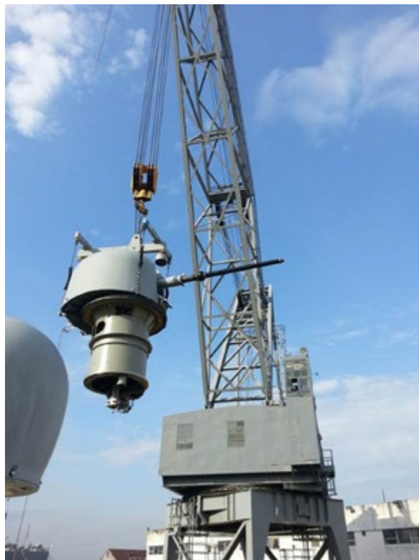
An MK 75, 76mm/62 caliber gun mount is removed from one of five U.S. Navy frigates being harvested by Engineers at Naval Ship Systems Engineering Station, Naval Surface Warfare Center Carderock Division (NAVSSES) in conjunction with the Naval Sea Systems Command (NAVSEA) Surface Warfare Directorate (SEA 21). The gun mount was supplied to the U.S. Coast Guard for use on their cutters. (U.S. Navy photo by Ashley Ferguson/Released)
