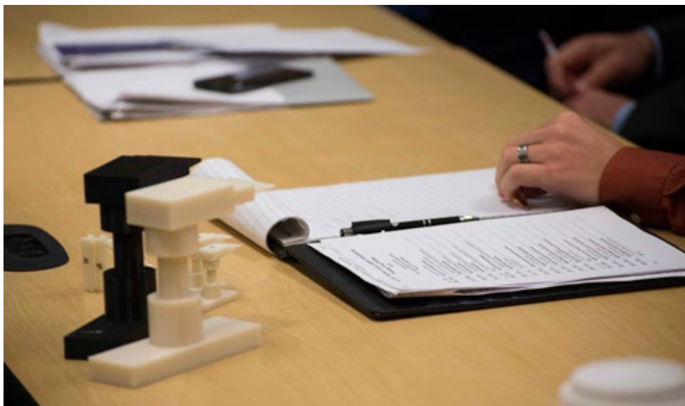
3-D printed test objects displayed at the additive manufacturing working group held Sept. 24-25, 2014, at Naval Surface Warfare Center, Carderock Division, West Bethesda, Md. The samples shown were produced during recent motion tests. They demonstrate variances that occur when printing objects while subjected to movements similar to conditions found on a ship at sea. (U.S. Navy photo by Nick Malay/Released)
