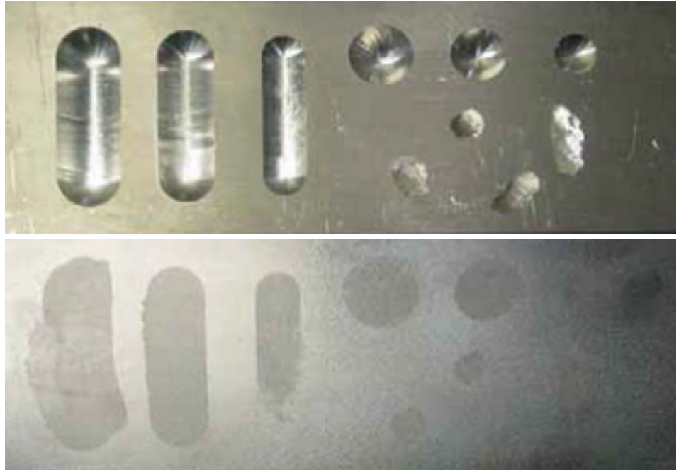
Top: Aluminum test plate before application of repair material using cold spray equipment. Bottom: Aluminum test plate after application of repair material using cold spray equipment and finishing using standard grinding and polishing techniques. (Photo courtesy of Innovative Materials and Processing Team, U.S. Army Research Laboratory/Released)
