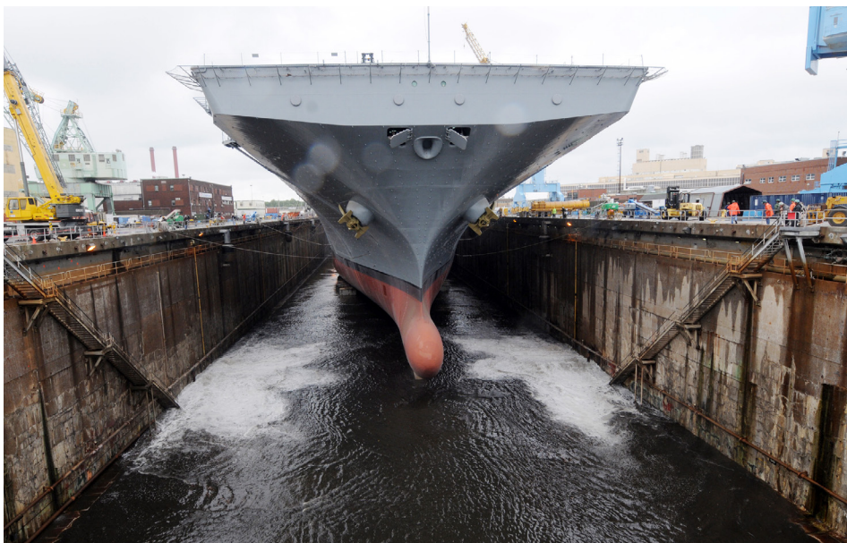
The amphibious assault ship USS Kearsarge (LHD 3) during a dry dock flooding operation at Norfolk Naval Shipyard, Sept. 8, 2009. (U.S. Navy photo by Mass Communication Specialist 1st Class Emmitt J. Hawks/Released)
