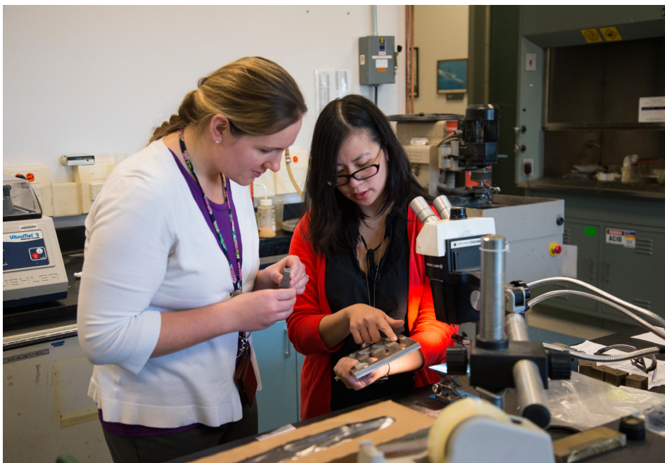
Dr. Jennifer Wolk (right) and Susan Hovanec discuss the shear and bonding characteristics of a cold spray material sample at Naval Surface Warfare Center, Carderock Division. The materials are being studied to confirm the reliability of cold spray repairs for both naval aircraft and ships. Their collaboration produced results that provide significant savings in both time and money in areas beyond Navy air and ship repairs. (U.S. Navy photo by Timothy E. Hunt/Released)
