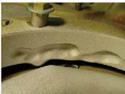
The UH-60 Lubricant Sump (shown) is cast from magnesium and is commonly affected by corrosion. Army and Navy rotorcraft and Air Force fighters each have 20 or more magnesium parts. Considering 4,550 rotorcraft in the Army and Navy inventory and up to 20 percent of the inventory typically affected at any one time by this issue, cold spray technologies can have a large impact on readiness. (Photo courtesy of Innovative Materials and Processing Team, U.S. Army Research Laboratory/Released)
