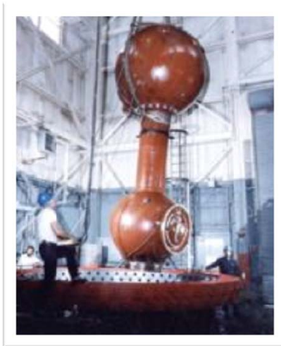
Hull Pressure Testing
