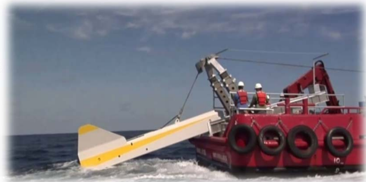
Contractor Testing of the EMM PPTA to test end-to-end L&R and tow operations prior to contract award
