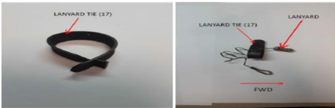
Picture 2. Lanyard Tie and Emergency/O2 Lanyard
